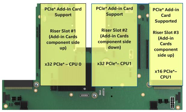
Figure 48. PCIe\* Add-in Card Orientation
