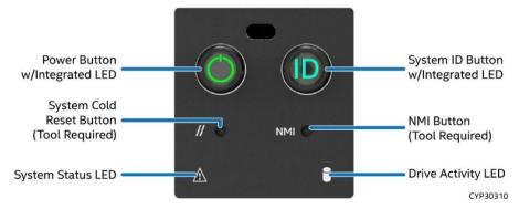
Figure 118. Front Control Panel Features
