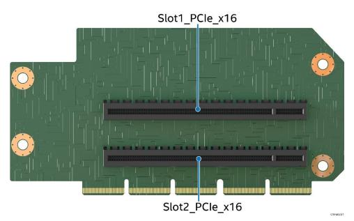
Figure 55. Two-Slot PCIe\* Riser Card for Riser Slot #1
