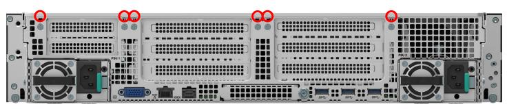
Figure 23. Rear Panel Shipping Screw Holes
