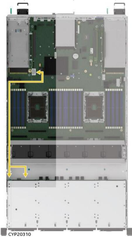
Figure 57. Cable Routing Between PCIe\* NVMe\* Riser Card and HSBP
