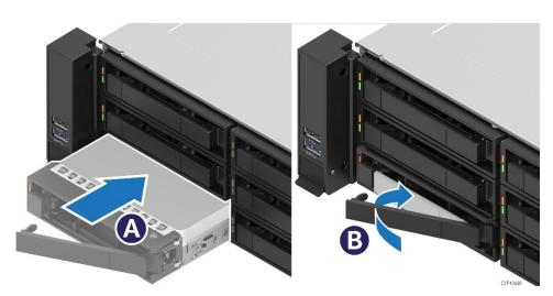
Figure 80. Drive Insertion into 3.5" Drive Bay
