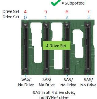
Figure 103. Supported Drive Population for Server Board SlimSAS Connectors or Tri-Mode Intel® RAID Module
