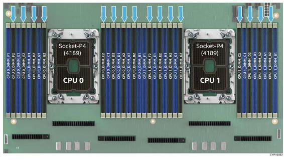
Figure 40. System DIMM / DIMM Blanks Configuration
