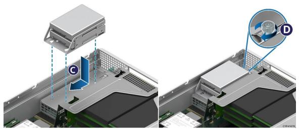
Figure 116. 2.5" Solid State Drive (SSD) Mounting Option
