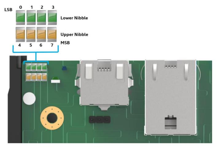
Figure 132. Server Board POST Diagnostic LEDs
