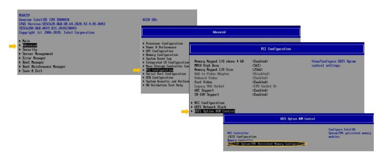
Figure 30. <F2> BIOS Setup Screen Navigation for Intel® Optane™ PMem Setup Options
