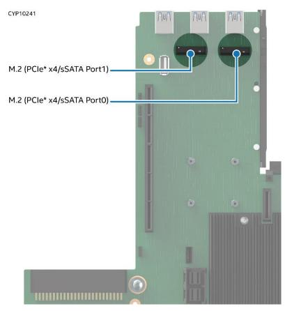
Figure 115. M.2 Module Connector Location
