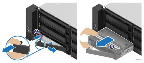
Figure 81. Drive Removal from 3.5" Drive Bay
