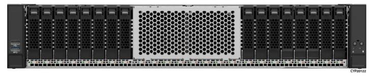
Figure 7. 16 x 2.5" Front Drive Bay Configuration (based on M50CYP2UR208)
