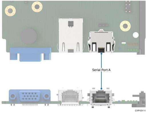
Figure 122. Serial Port A
