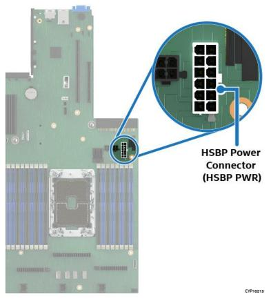
Figure 87. Server Board HSBP Power Connector
