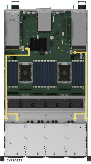
Figure 22. System Cable Routing Channels
