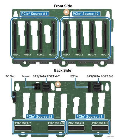
Figure 102. Backplane Cabling from Two Backplane Sources
