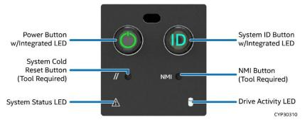
Figure 5. Front Control Panel Feature Identification
