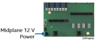
Figure 96. Midplane 12 V Power Connector on Server Board
