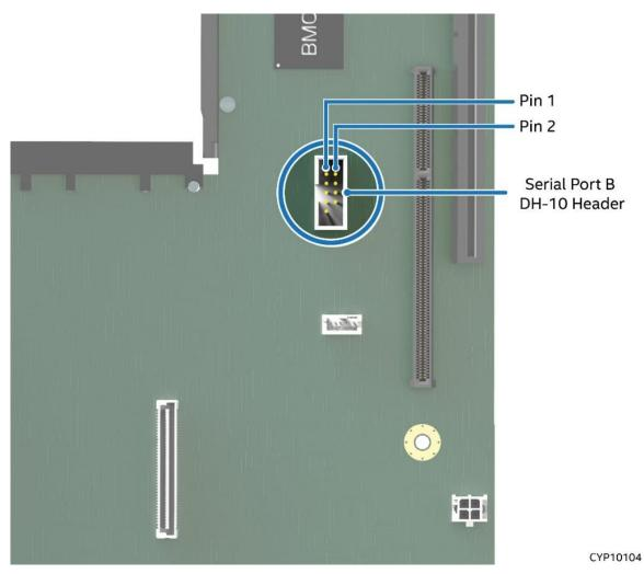
Figure 125. Serial Port B Header (Internal)
