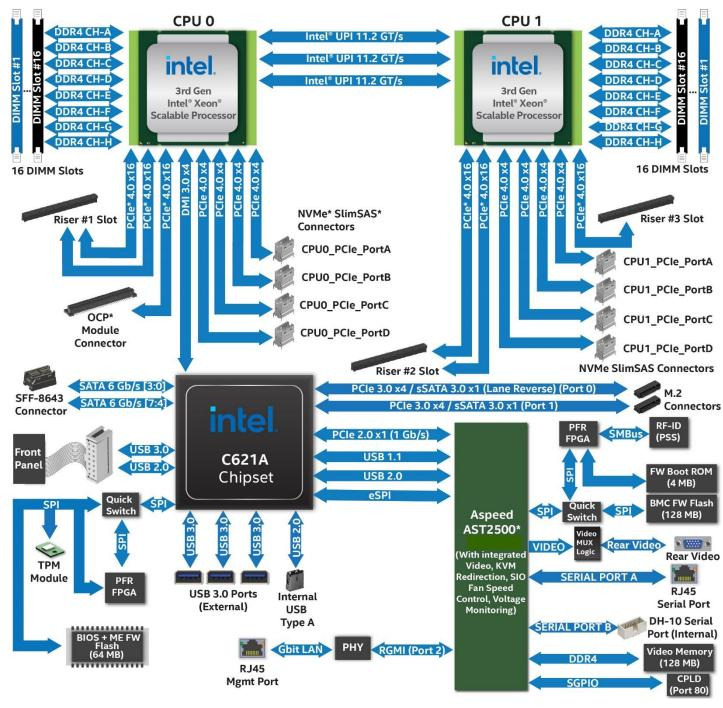
Figure 10. Intel® Server Board M50CYP2SBSTD Architectural Block Diagram
