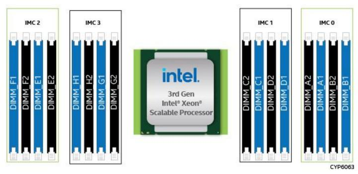
Figure 33. Memory Slot Identification
