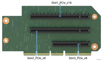
Figure 54. PCIe\* Riser Card for Riser Slot #1
