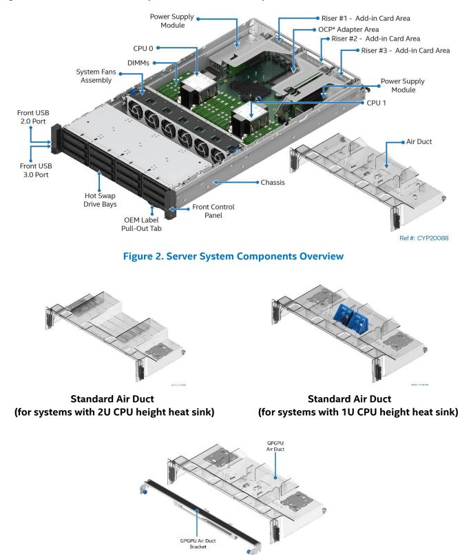
GPGPU Air Duct (for systems with 1U CPU height heat sink and GPGPU add-in card)
