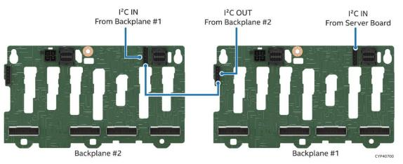
Figure 90. Connecting Two x8 Backplanes
