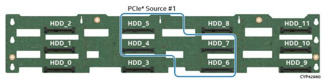
Figure 105. 12 x 3.5" HSBP NVMe\* Connector Identification – Front Side
