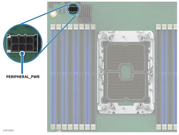
Figure 117. Peripheral Power Connector Identification
