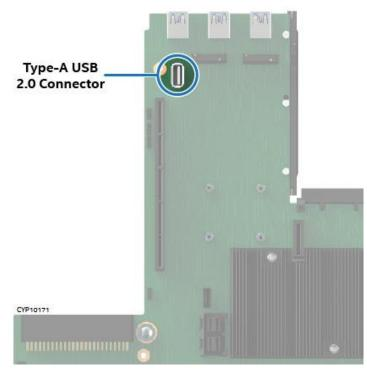
Figure 127. Internal USB 2.0 Type-A Connector Table 61. Internal USB 2.0 Type-A Connector Pinout
