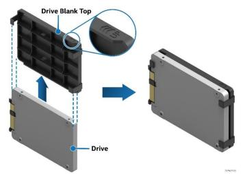
Figure 71. 2.5" 7 mm Height Drive Insertion using Drive Blank
