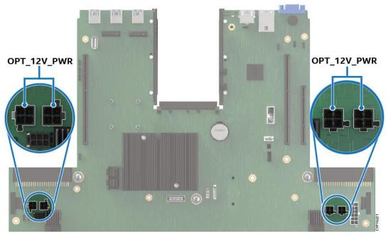
Figure 61. Riser Slot Auxiliary Power Connectors
