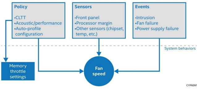
Figure 42. High Level Fan Speed Control Structure
