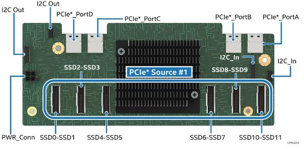
Figure 104. Drive Set and Connector Identification
