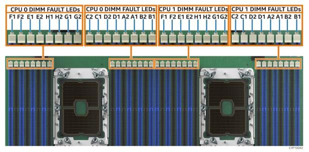
Figure 130. Memory Fault LED Location
