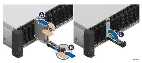
Figure 73. 7 mm Drive Insertion into 2.5" Drive Bay
