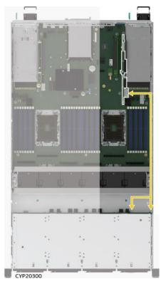
Figure 99. Cable Routing Between PCIe\* NVMe\* Riser Card and HSBP 8.2.2.2 PCIe\* NVMe\* Riser Card for Riser Slot #1 (iPC – CYP2URISER1RTM)
