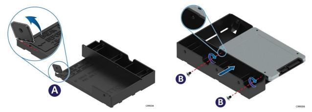
Figure 82. 2.5" SSD Installation into Drive Blank – Tab Removal and SSD Insertion
