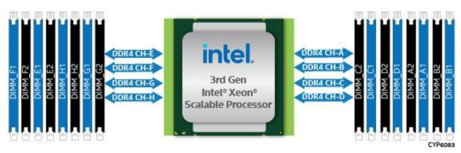
Figure 27. Memory Slot Connectivity
