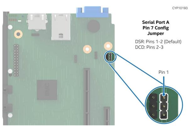
Figure 124. J19 Jumper Header for Serial Port A Pin 7 Configuration
