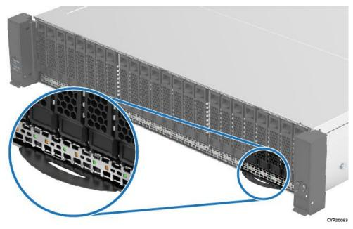
Figure 17. Pull-out Tab Location
