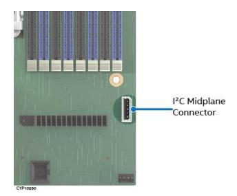
Figure 95. I<sup>2</sup>C Midplane Connector on Server Board
