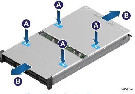
Figure 20. System Top Cover Removal
