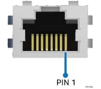
Figure 123. RJ45 Serial Port A Connector Pin Orientation
