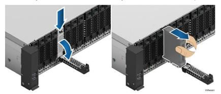
Figure 74. 7 mm Drive Removal from 2.5" Drive Bay
