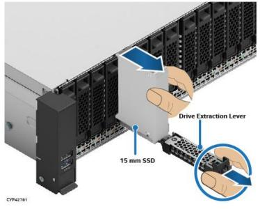
Figure 77. 15 mm Drive Removal from 2.5" Drive Bay
