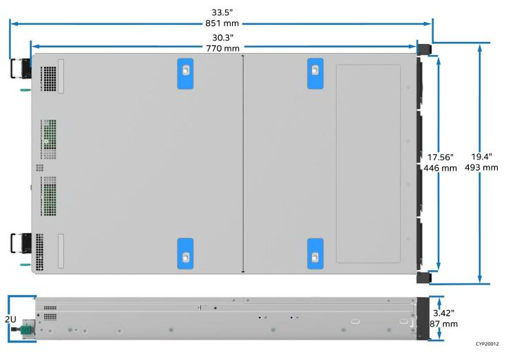
**Figure 15. Chassis Dimensions**
