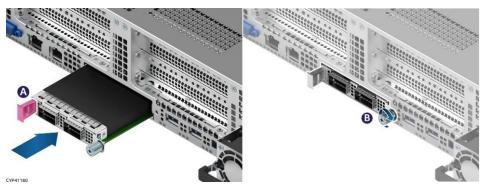
Figure 64. OCP\* Adapter with Pull tab Installation
