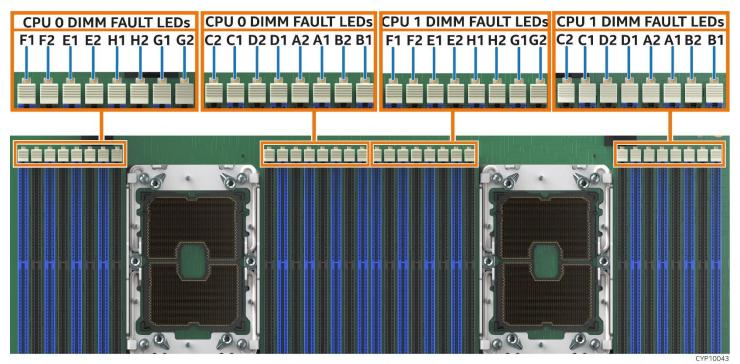
Figure 13. Intel<sup>®</sup> Light-Guided Diagnostics - DIMM Fault LEDs
