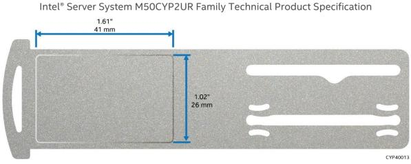
Figure 18. Pull-out Tab Label Emboss Dimensions
