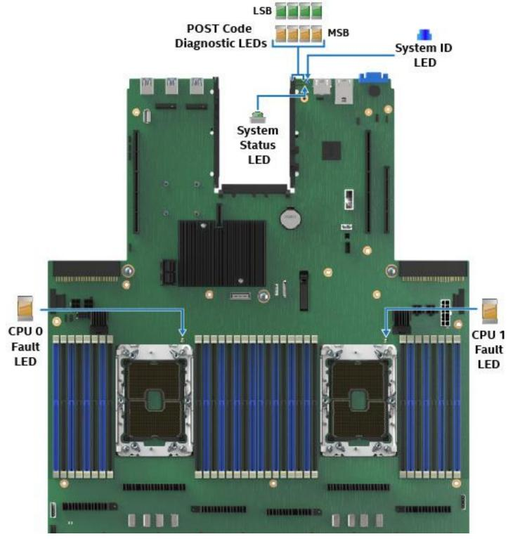
Figure 12. Intel<sup>®</sup> Light-Guided Diagnostics – LED Identification
