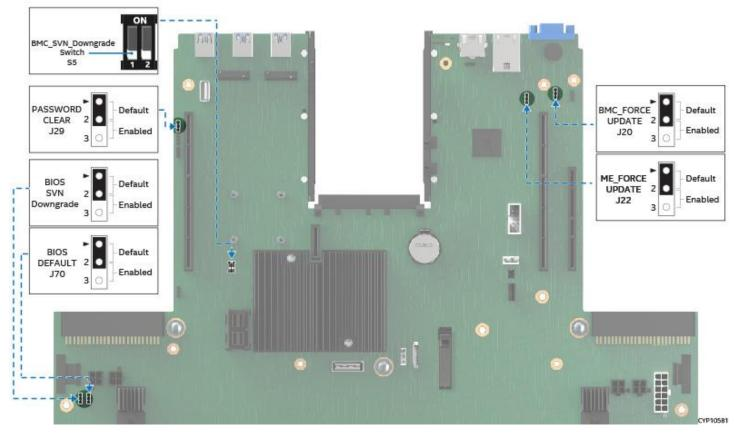
Figure 14. System Configuration and Recovery Jumpers
