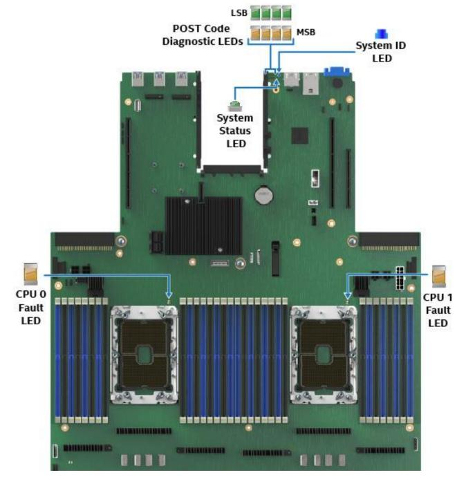
Figure 128. Intel® Server System M50CYP2UR Family LEDs
