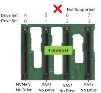
Mixing of NVMe\* and SAS within a common drive set is not supported
