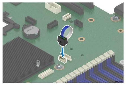
Figure 101. Intel<sup>®</sup> VROC 7.5 Key Insertion
