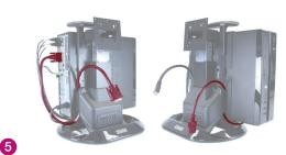
Secure the PC receiving frame to the stand using two #6-32 hex socket screw in the
