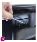
Lock the monitor to the UniStand using a single M4 6mm hex socket screw.
