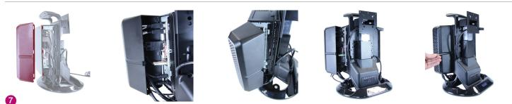
Attach the cable management cover to the PC receiving frame by hooking it into position on the three protruding tabs, then rotating it on the hinged axis. Ensure that when closing the cover over the cables, no undue stress is placed on the connectors. Once fully closed, lock the cover in position with a single #6-32 hex socket screw.
