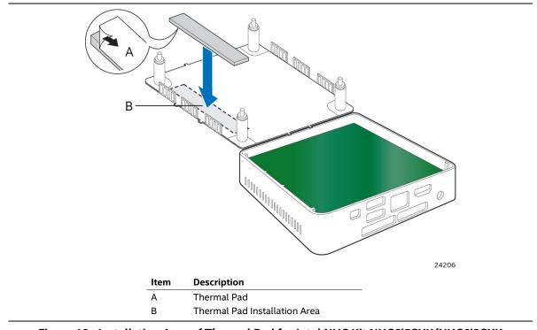
Figure 19. Installation Area of Thermal Pad for Intel NUC Kit NUC6i5SYK/NUC6i3SYK
