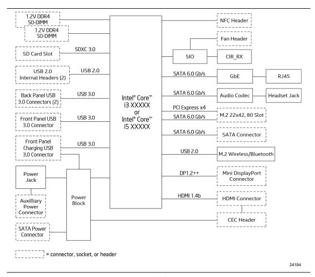
Figure 3. Block Diagram
