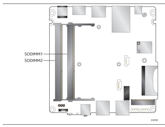
Figure 4. Memory Channel and SO-DIMM Configuration
