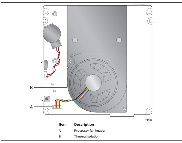
Figure 7. Thermal Solution and Fan Header
