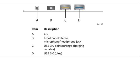
Figure 9. Front Panel Connectors
