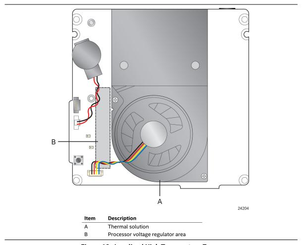
Figure 18. Localized High Temperature Zones
