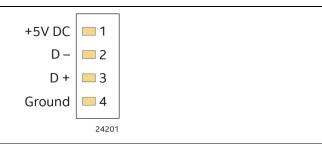
Figure 13. Connection Diagram for Internal USB 2.0 Single-Port Header (1.25 mm Pitch)
