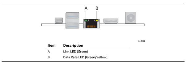
**Figure 6. LAN Connector LED Locations**
