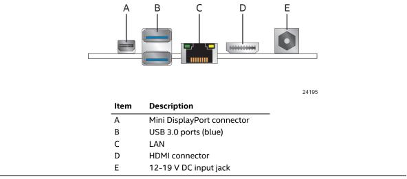
Figure 10. Back Panel Connectors
