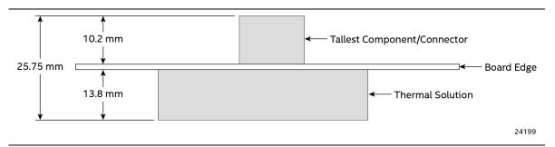
Figure 17. Board Height Dimensions
