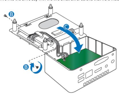
4. Set the drive bay bracket down inside the chassis (C), taking care not to pinch the SATA cables along the edge.
