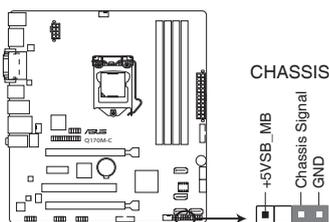
**Q170M-C Chassis intrusion connector**
