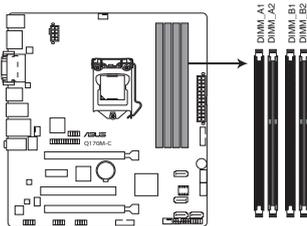
Q170M-C 288-pin DDR4 DIMM sockets
