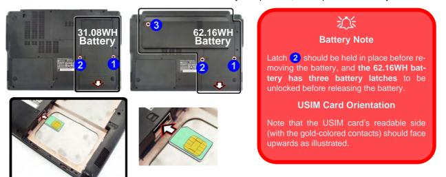
Figure 1 - 7 - Battery Removal & USIM Card Installation
