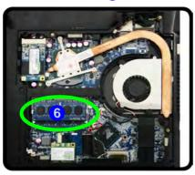
Gently pull the two release latches on the sides of the memory socket in the direction indicated by the arrows (7 & 8) in *Figure 6 - 9*.
