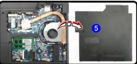
Figure 6 - 8 Removing the Component Bay Cover
