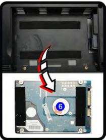
Figure 6 - 3 Hard Disk Assembly Removal
