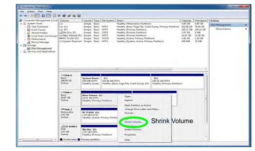
Figure 7 - 31 Computer Management (Shrink SSD Volume) 4. Enter the figure, which should be equal to amount of system memory (RAM) in your computer, in "Enter the amount of space to shrink in MB".
