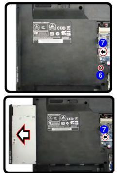
*Figure 6 - 6* Removing the Optical Device Drive (Model A)
