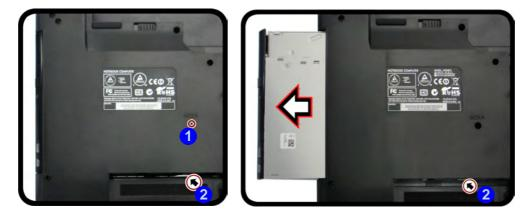
*Figure 6 - 7* Removing the Optical Device Drive (Model B)
