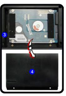
*Figure 6 - 2* Hard Disk Bay Cover Removal
