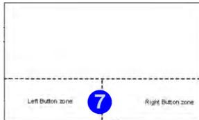
Note that the Touchpad and Buttons has a valid operational area indicated within the dotted lines above.
