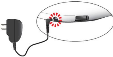
While the system is off, it takes at least 4hrs to fully charged the battery.
