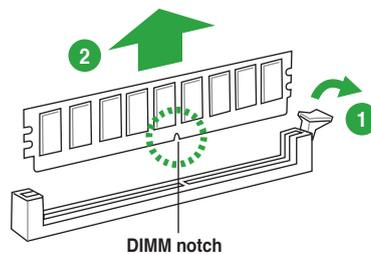
2. Remove the DIMM from the socket.
