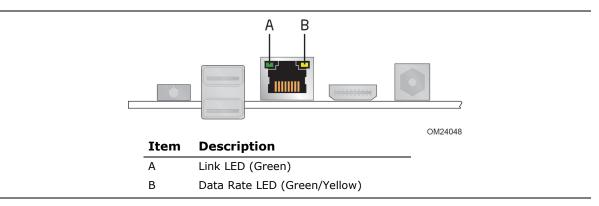
**Figure 6. LAN Connector LED Locations**
