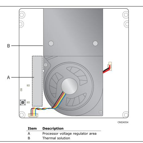
Figure 16. Localized High Temperature Zones
