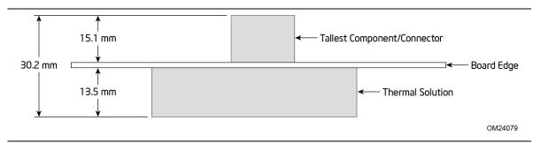
Figure 15. Board Height Dimensions
