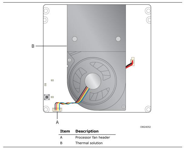
Figure 7. Thermal Solution and Fan Header
