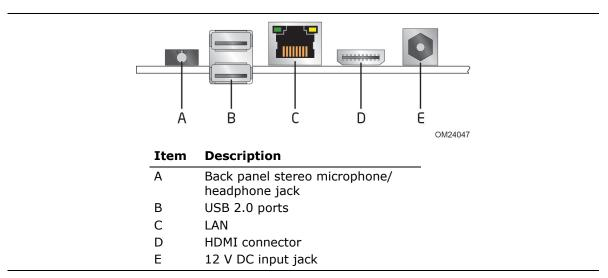
Figure 10. Back Panel Connectors
