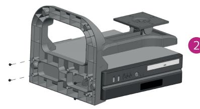
Secure the chassis and foot stand together using 4 screws (supplied).
