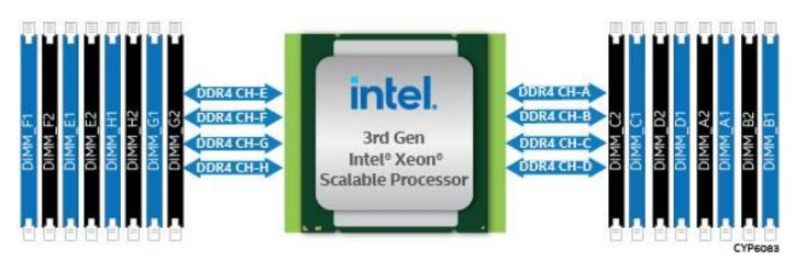
Figure 20. Memory Slot Connectivity
