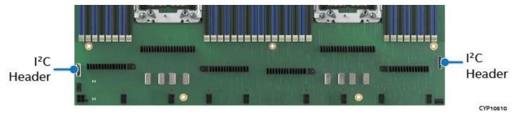
Figure 38. I<sup>2</sup>C Connectors
