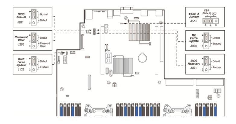
Figure 7. System Configuration and Recovery Jumpers
