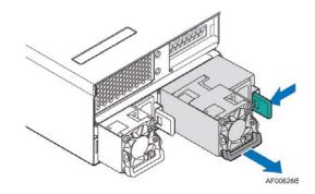
Figure 25. Power Supply Module Identification
