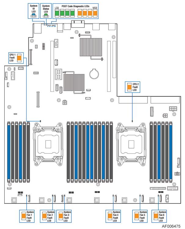
Figure 5. Light Guided Diagnostic LEDs
