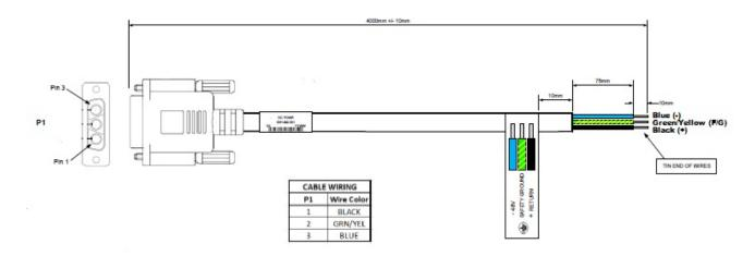
Figure 29. DC Power Cord Specification
