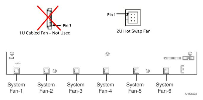
Figure 32. Server Board 2U System Fan Connector Locations
