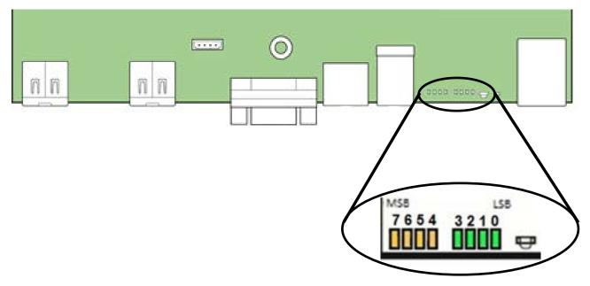
Figure 82. POST Diagnostic LED Location
