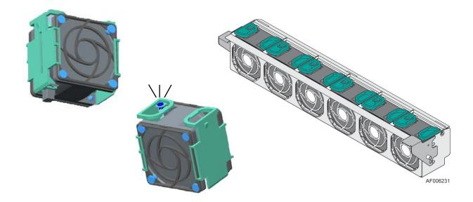
Figure 33. System Fan Assembly
