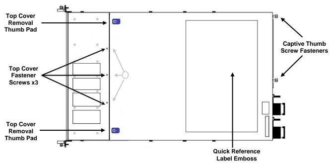
Figure 3. 2U Top Cover Features - (System with 12 x 3.5" Drive Bay)
