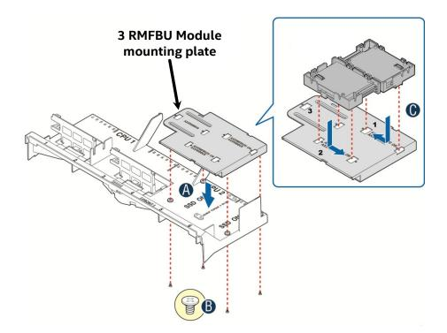
Figure 68. Triple RMFBU (Default) Mounting Bracket Installation
