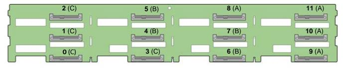
Note: Letters in parenthesis denote references to connectors on the backside of the backplane as illustrated in the following diagram
