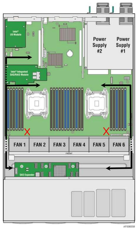
Figure 24. System Cable Routing Channels
