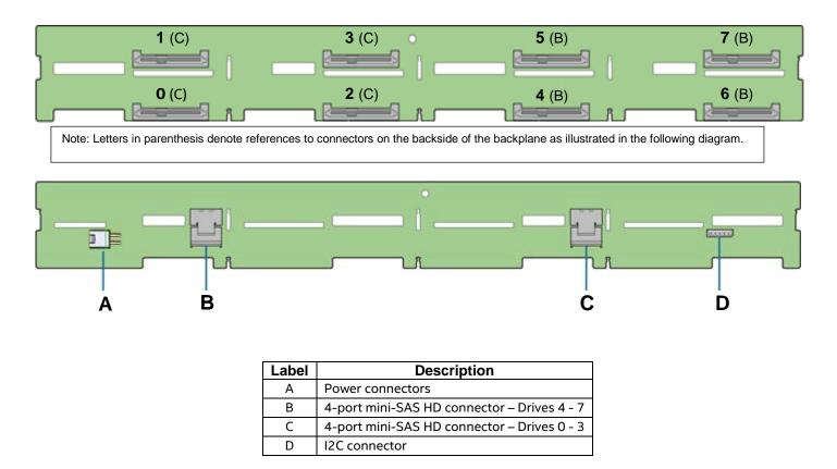
Figure 60. 8 x 3.5" HSBP Connector Identification
