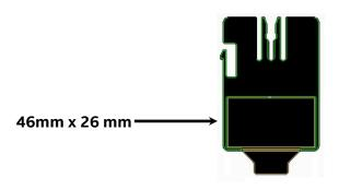
Figure 22. Pull-out Tab Label Emboss Dimensions – Non-Storage Models
