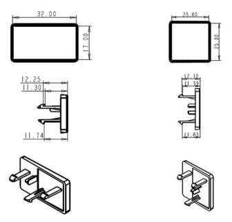
Figure 19. Front Bezel accesssory ID Badge mechanical drawings
