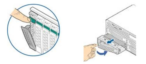
There are drive carriers to support 2.5" devices and 3.5" devices. To maintain system thermals, all drive bays must be populated with a drive carrier mounted with a hard disk drive, SSD, or supplied drive blank.
