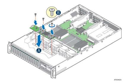
In the 2U 12x3.5" system configuration, the SAS expander must be installed in any available PCIe add-in slot.
