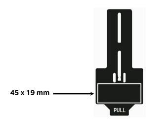
Figure 23. Pull-out Tab Label Area Dimensions – Storage Models
