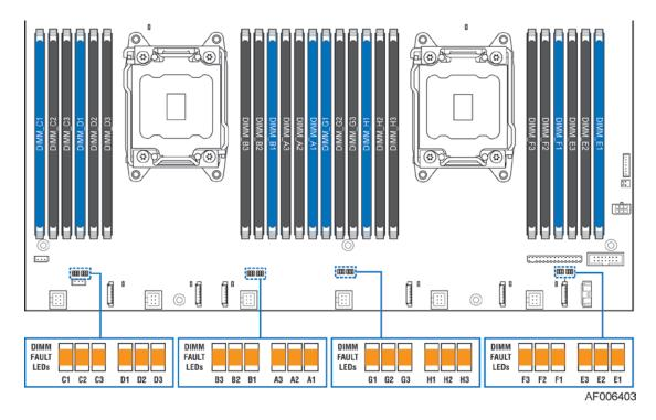
Figure 6. DIMM Fault LEDs
