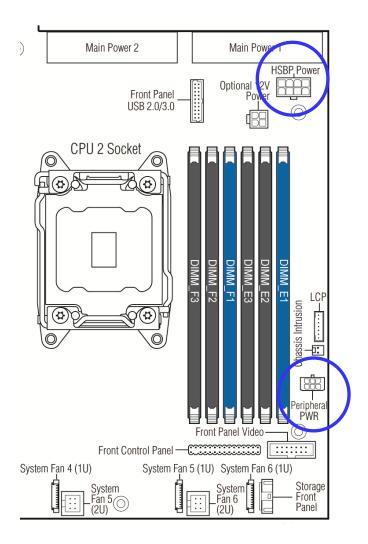
Figure 44. Server Board Peripheral Power Connectors
