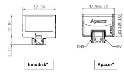
Each installed SATA DOM plugs directly into one of the white single port SATA connectors on the server board, which provide both power and I/O signals.
