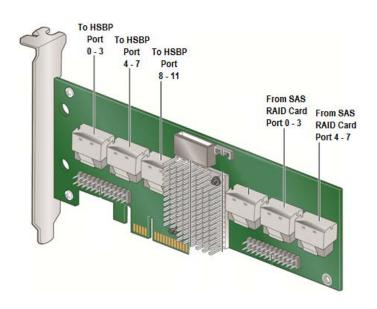
Figure 71. Intel® RAID Expander RES2SV240 Connector Identification
