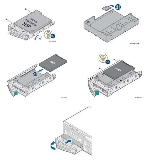
Note: Due to degraded performance and reliability concerns, the use of the 3.5" drive blank as a 2.5" device bracket is intended to support SSD type storage devices only. Installing a 2.5" hard disk drive into the 3.5" drive blank cannot be supported.
