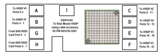
Figure 72. – 12Gb Internal 36-Port Intel® RAID Expander Card RES3TV360 - Connector Identification Block Diagram
