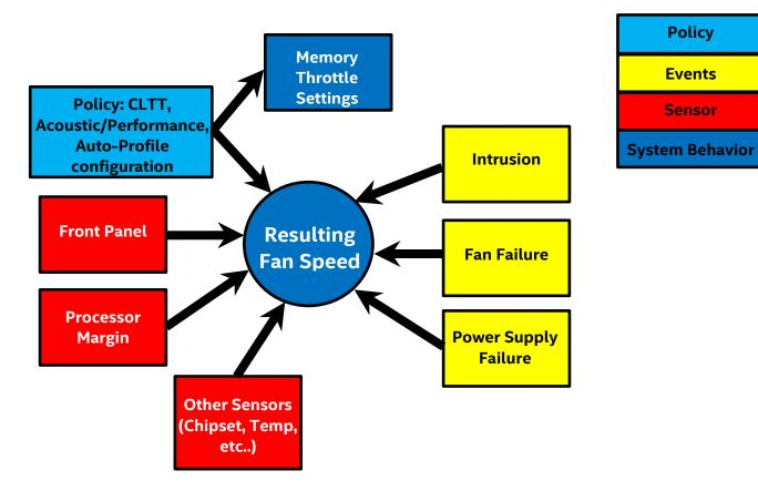
Figure 31. Fan Control Model
