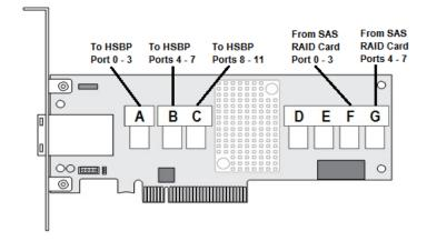
Figure 70. Intel® RAID Expander RES3FV288 Connector Identification
