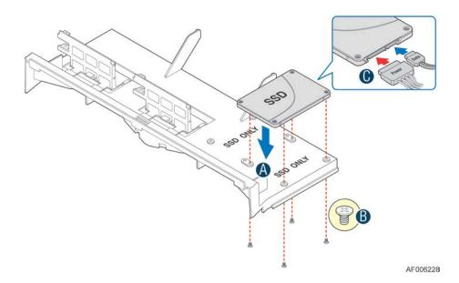
Figure 63. 2.5" Solid State Drive (SSD) Mounting Option
