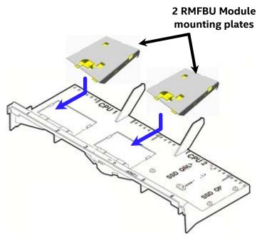
Figure 69. Dual RMFBU Mounting Bracket Installation
