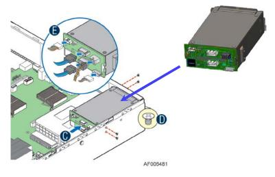
Figure 61. 2 x 2.5" Rear Mount Backplane Kit Placement
