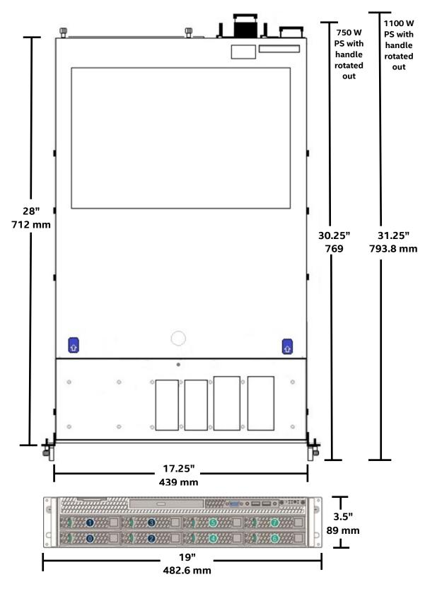
Figure 20. Chassis Dimensions
