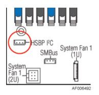
Figure 57. "HSBP\_I2C" connector on the server board
