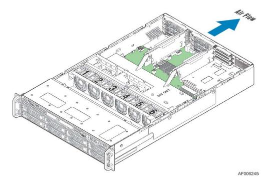
Figure 30. System Air Flow and Fan Identification
