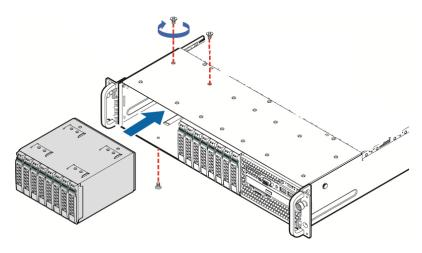
Figure 48. 2.5" Drive Bay Module Placement
