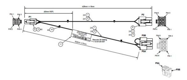
Figure 35. Auxiliary 12V Power Cable (iPC AXXGPGPUCABLE)
