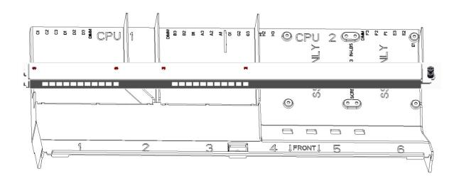
Figure 38. Shipping Bracket Placement
