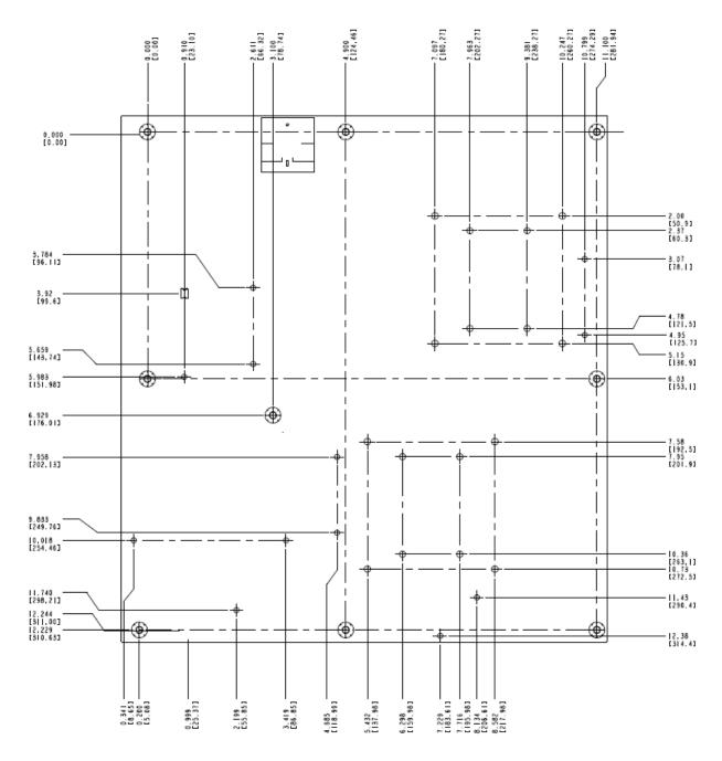
Figure 4. Intel<sup>®</sup> Server Board S2400GP – Mounting Hole Locations (1 of 2)
