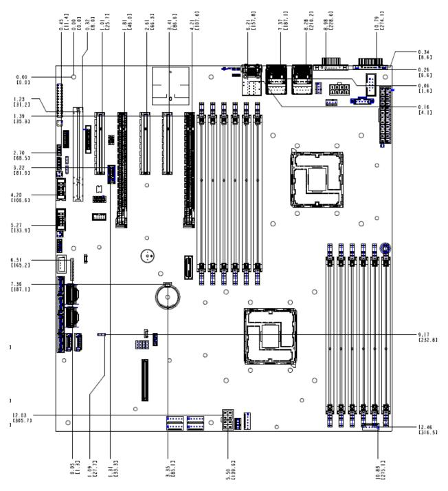
Figure 7. Intel<sup>®</sup> Server Boards S2400GP – Major Connector Pin-1 Locations (2 of 3)
