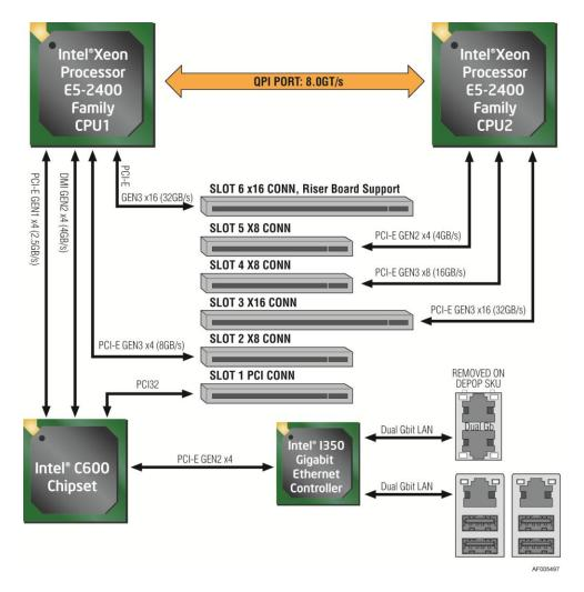
Figure 16. Functional Block Diagram of Processor IIO Sub-system
