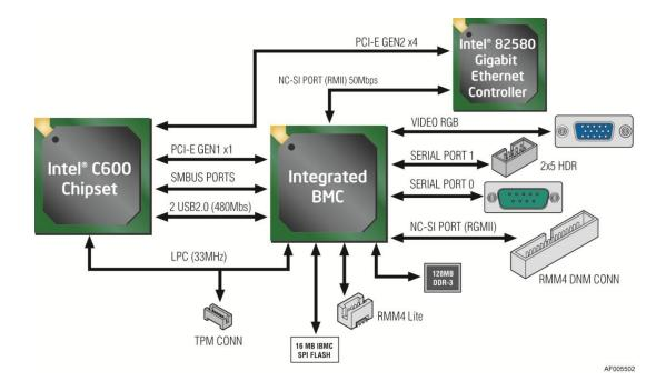
Figure 18. Integrated Baseboard Management Controller (BMC) Overview
