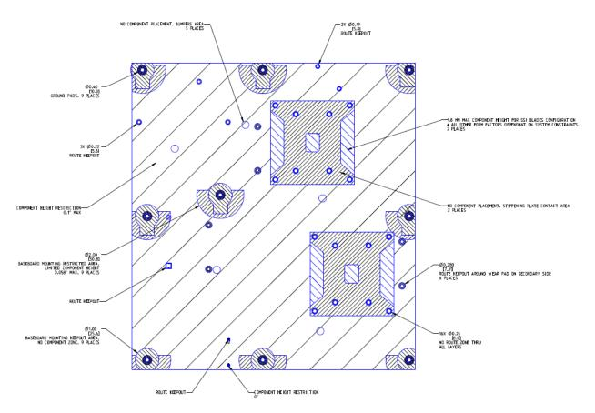
Figure 11. Intel<sup>®</sup> Server Boards S2400GP – Second Side Keep-out Zone
