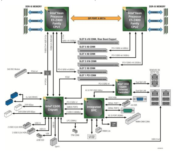
Figure 13. Intel® Server Board S2400GP Functional Block Diagram
