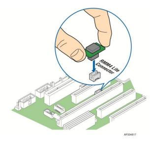
Figure 22. Intel<sup>®</sup> RMM4 Lite Activation Key Installation
