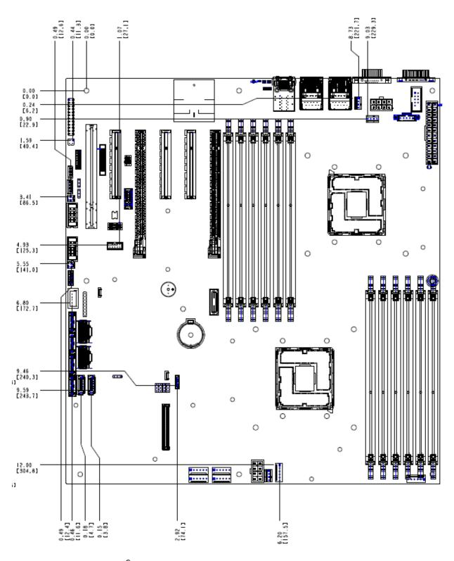
Figure 8. Intel<sup>®</sup> Server Boards S2400GP – Major Connector Pin-1 Locations (2 of 3)
