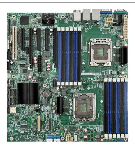
Figure 1. Intel<sup>®</sup> Server Board S2400GP Layout (S2400GP4 as example)
