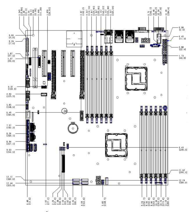
Figure 6. Intel<sup>®</sup> Server Boards S2400GP – Major Connector Pin-1 Locations (1 of 3)
