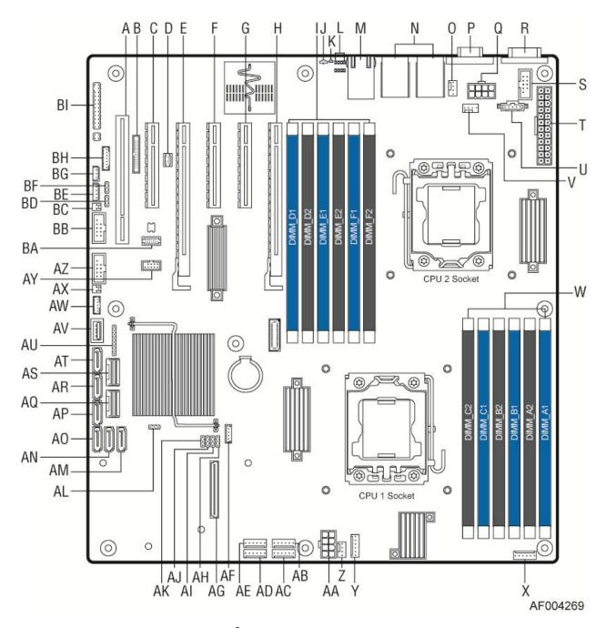
Figure 2. Intel<sup>®</sup> Server Board S2400GP Components
