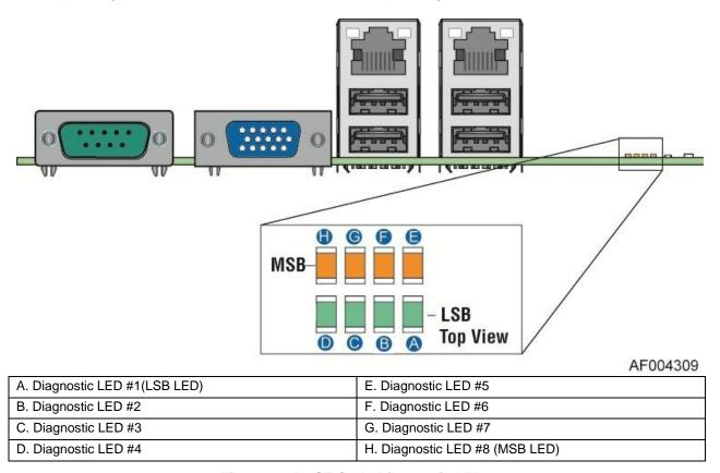
Figure 32. POST Code Diagnostic LEDs
