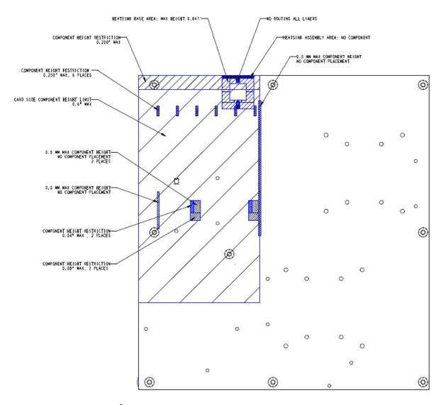
Figure 10. Intel<sup>®</sup> Server Boards S2400GP – Primary Side Card Side Keep-out Zone
