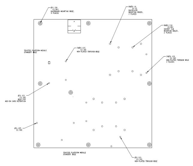
Figure 5. Intel<sup>®</sup> Server Board S2400GP – Mounting Hole Locations (2 of 2)
