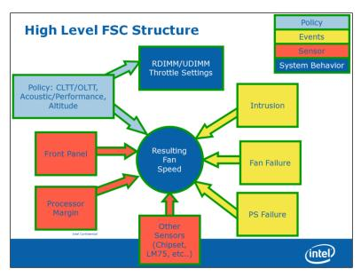
Figure 21. Fan Speed Control Process
