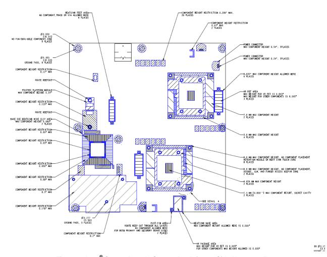
Figure 9. Intel<sup>®</sup> Server Boards S2400GP – Primary Side Keep-out Zone
