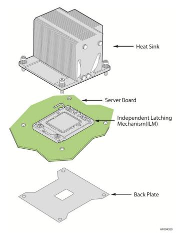
Figure 14. Processor Socket Assembly
