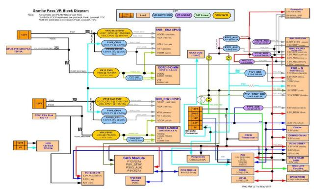
Figure 31. Power Distribution Block Diagram
