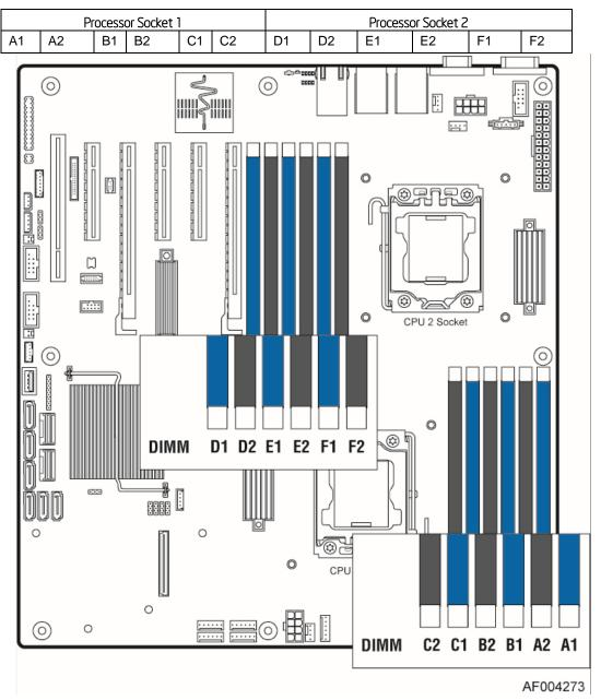
Figure 15. Intel® Server Board S2400GP DIMM Slot Layout
