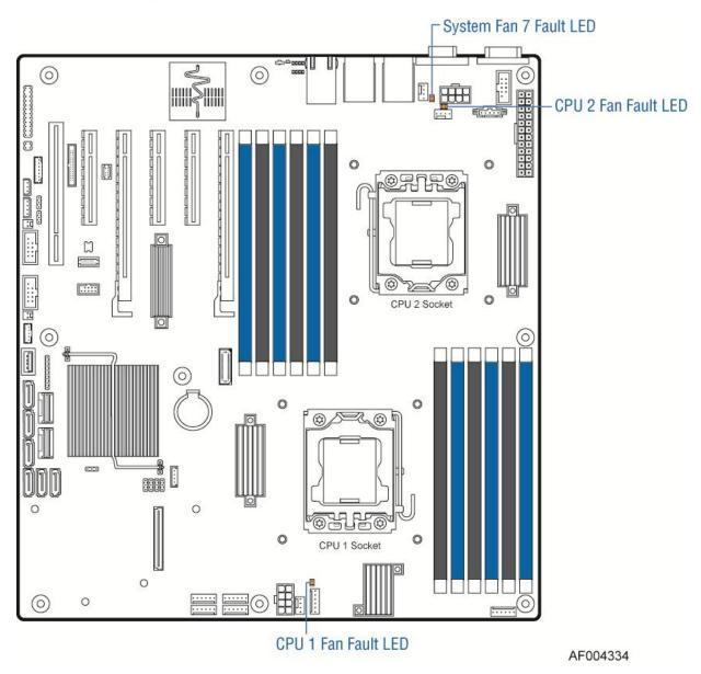
Figure 26. Fan Fault LED Locations
