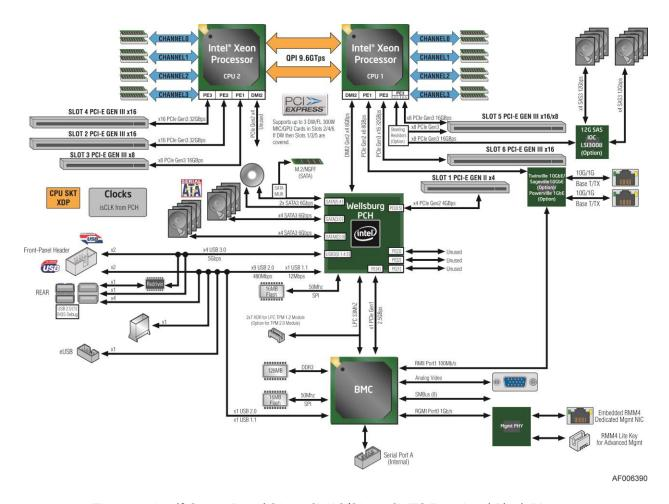
Figure 12. Intel® Server Board S2600CW2S/S2600CWTS Functional Block Diagram
