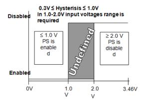
Figure 29. PSON# Required Signal Characteristic
