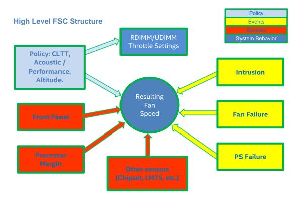
Figure 18. High-level Fan Speed Control Process
