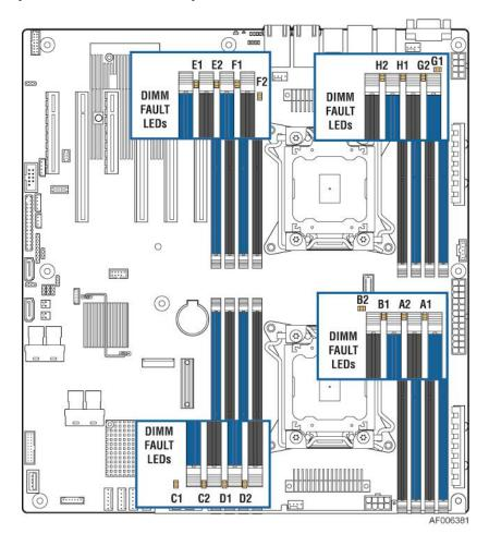
Figure 24. DIMM Fault LED's Location
