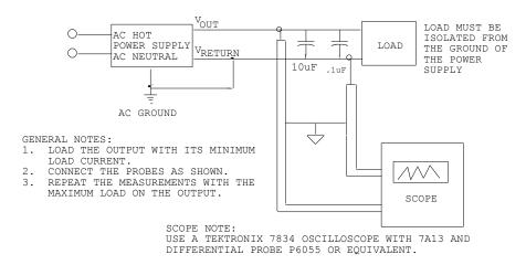
Figure 27. Differential Noise Test Setup
