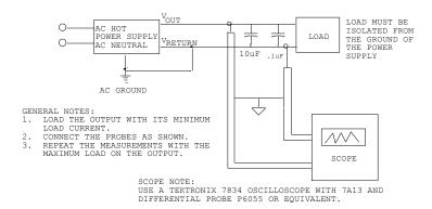
Note: When performing this test, the probe clips and capacitors should be located close to the load.
