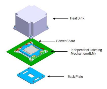
Figure 13. Processor Socket Assembly
