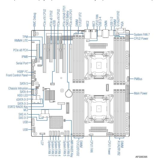
Figure 3. Connector and Component Layout
