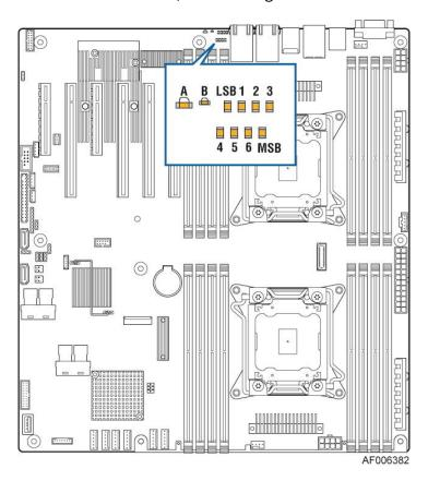
Figure 33. POST Code Diagnostic LED Decoder
