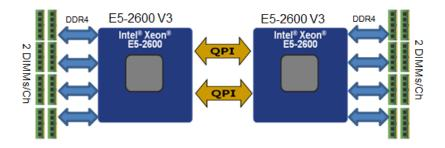
Figure 14. Memory Subsystem for Intel® Server Board S2600CW
