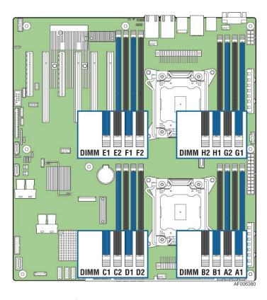
Figure 15. Intel® Server Board S2600CW DIMM Slot Layout
