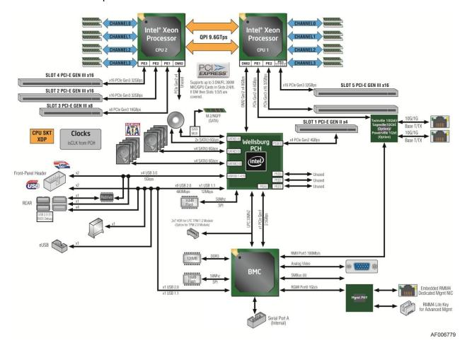
Figure 11. Intel® Server Board S2600CW2/S2600CWT Functional Block Diagram
