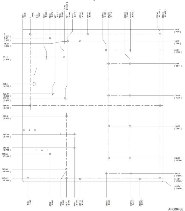
Figure 4. Mounting Hole Locations (1 of 2)
