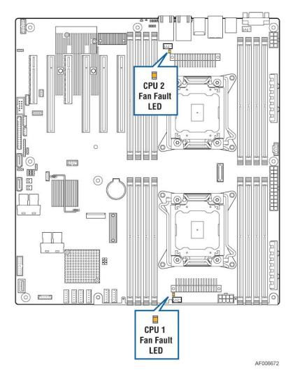
Figure 23. Fan Fault LED's Location
