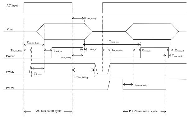
Figure 28. Turn On/Off Timing (Power Supply Signals)
