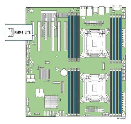
Figure 19. Intel® RMM4 Lite Activation Key Location
