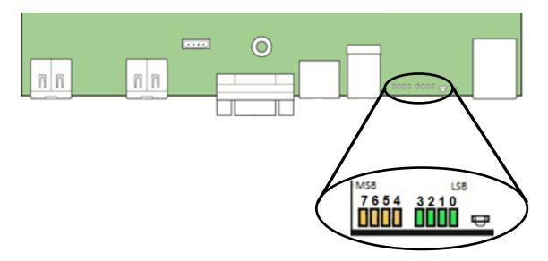
Figure 35. POST Diagnostic LED Location
