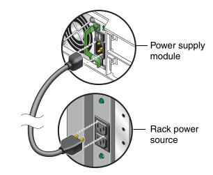
3. Connect the primary power cords from the rack to separate external power sources.
