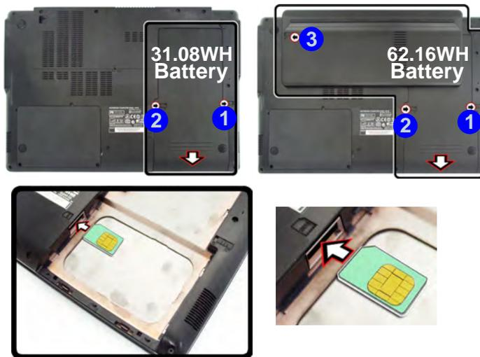
Figure 1 - 7 - Battery Removal & USIM Card Installation
