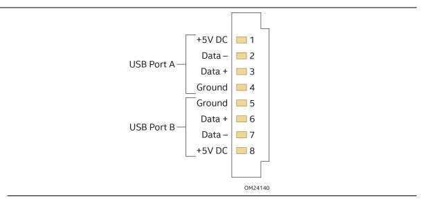
Figure 18. Connection Diagram for Internal USB 2.0 Dual-Port Header (1.25 mm Pitch)
