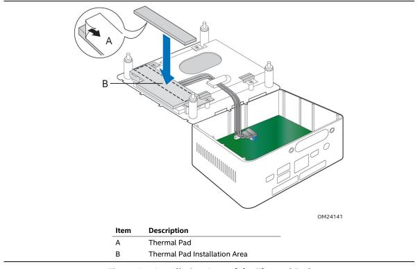
Figure 24. Installation Area of the Thermal Pad
