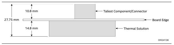
Figure 22. Board Height Dimensions
