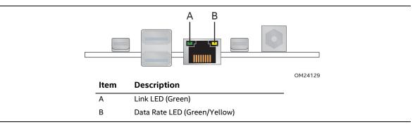
Figure 8. LAN Connector LED Locations
