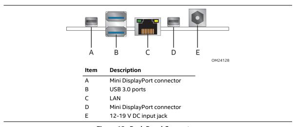
Figure 12. Back Panel Connectors
