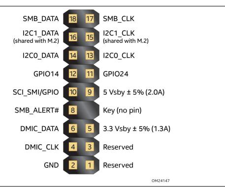
Figure 17. Low Speed Custom Solutions Header
