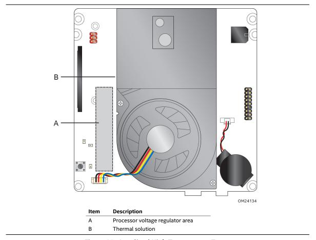
Figure 23. Localized High Temperature Zones
