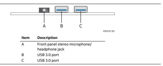
**Figure 11. Front Panel Connectors**
