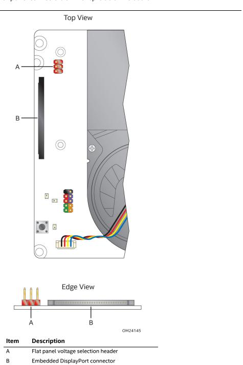
Figure 6. Flat Panel Connectors on Top-side of the Board
