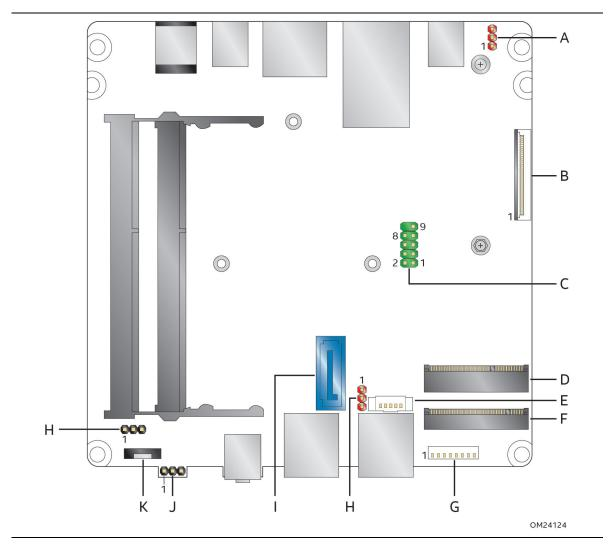
Figure 14. Connectors and Headers (Bottom)
