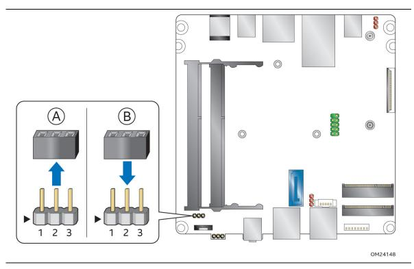
Figure 20. Intel MEBX Reset Header
