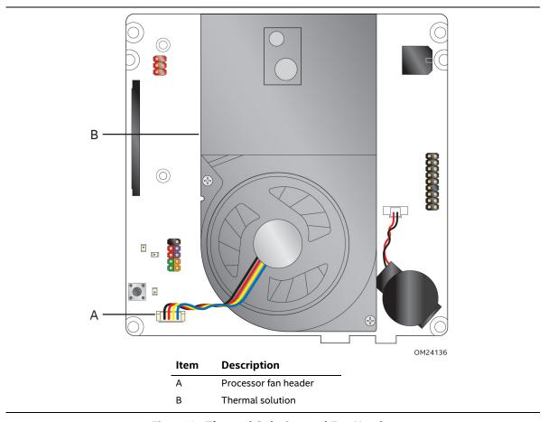
Figure 9. Thermal Solution and Fan Header
