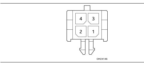
Figure 15. Connection Diagram for the Internal Power Supply Connector
