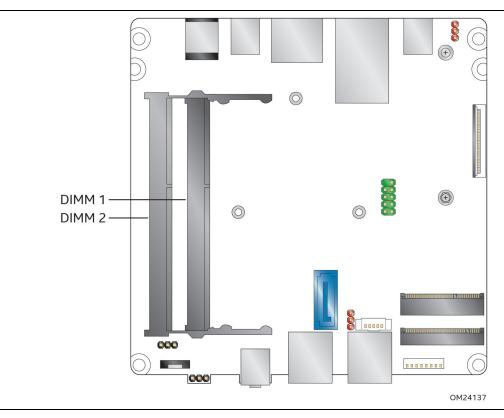
Figure 4. Memory Channel and SO-DIMM Configuration
