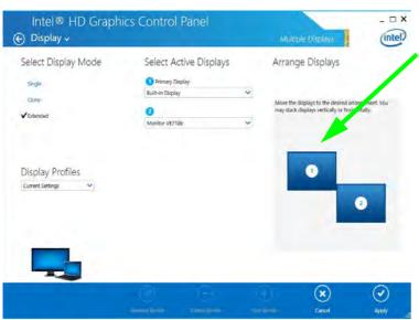
Click the appropriate monitor icon and drag it to match the physical arrangement you wish to use (e.g. the secondary display may be extended left/right/above/below the primary display).
