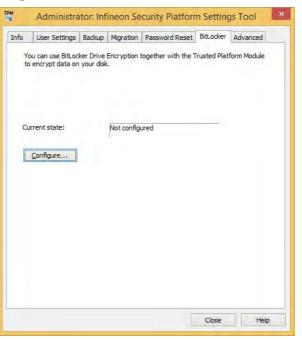
Access the Microsoft **BitLocker Drive Encryption** control panel applet from the *Windows* control panel (**System and Security**).
