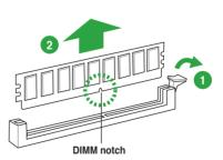
2. Remove the DIMM from the socket.
