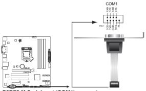
P8B75-M Serial port (COM1) connector
