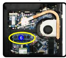
5. Gently pull the two release latches on the sides of the memory socket in the direction indicated by the arrows (7 & 8) in *Figure 6 - 8*.
