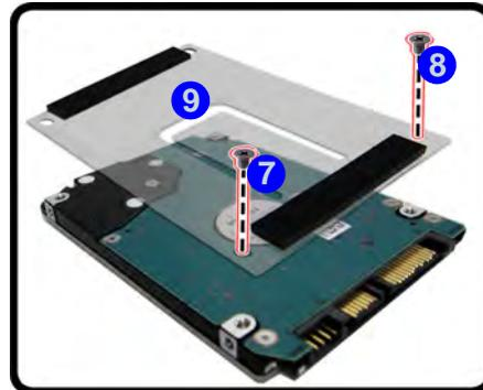
8. Reverse the process to install a new hard disk drive.
