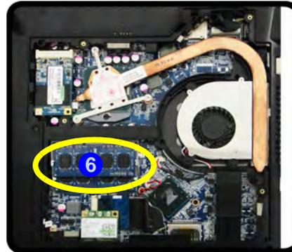
5. Gently pull the two release latches on the sides of the memory socket in the direction indicated by the arrows (⑦ & ⑧) in *Figure 6 - 8*.
