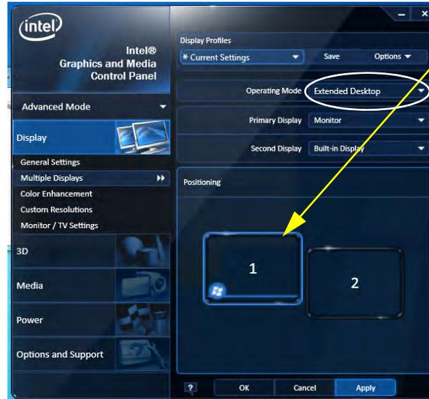
Click the appropriate monitor icon and drag it to match the physical arrangement you wish to use (e.g. the secondary display may be extended left/right/above/below the primary display).
