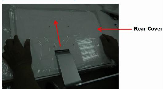
Step 3  $\rightarrow$  Rear Cover by sliding as direction as shown
