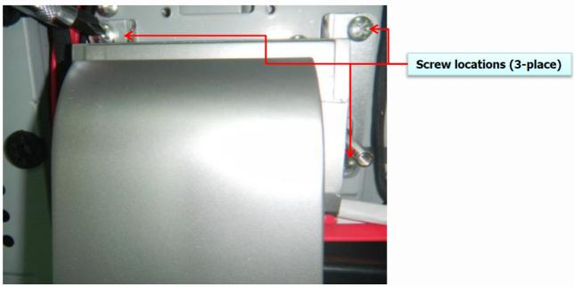
Step 2  $\rightarrow$  Remove L-Stand as direction as shown.
