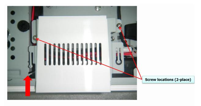
To install Rear small cover as direction as shown and fix it by 2 screws.
