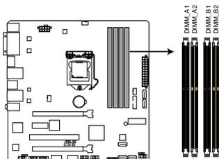
CS-B 240-pin DDR3 DIMM sockets
