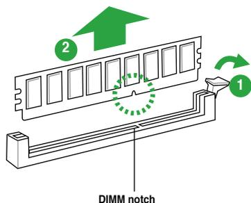
2. Remove the DIMM from the socket.
