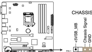
**CS-B Chassis intrusion connector**
