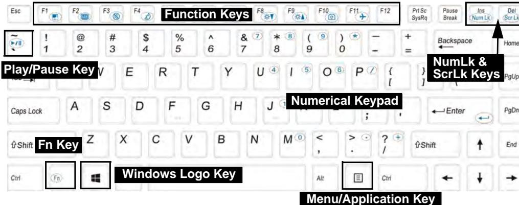
Figure 1 - 4 - Keyboard - Model A
