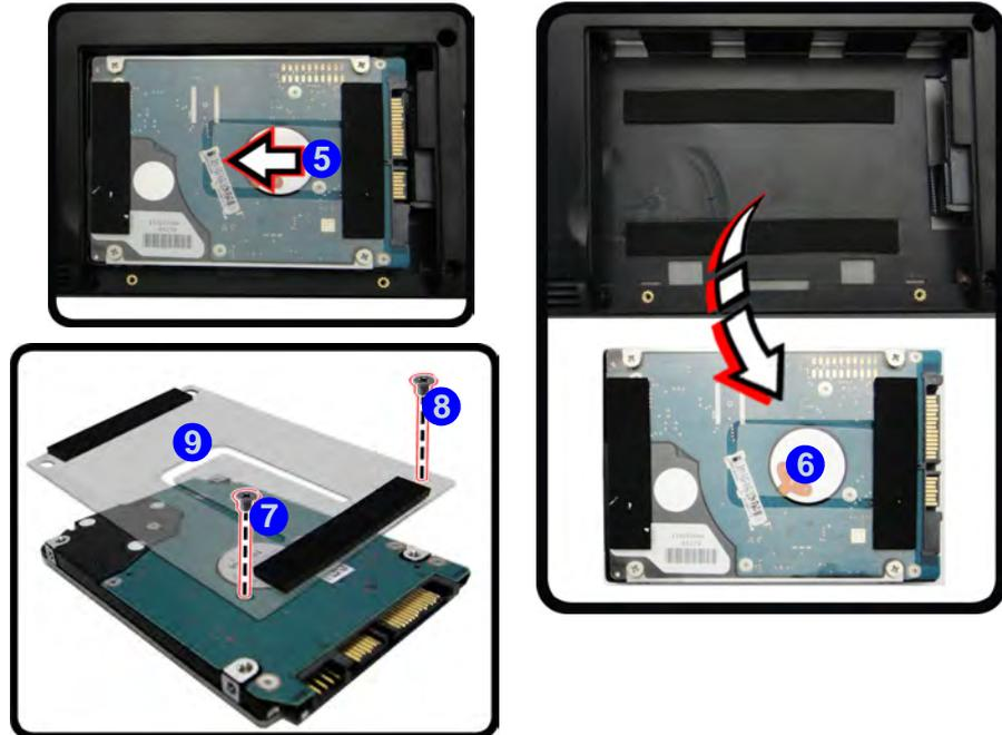
8. Reverse the process to install a new hard disk drive.
