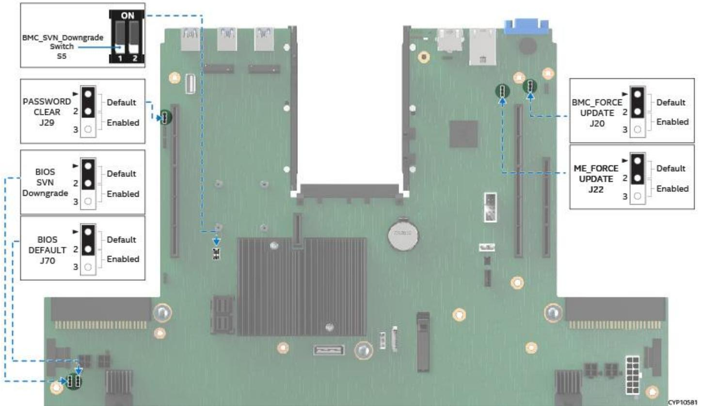
**Figure 7. System Configuration and Recovery Jumpers**
