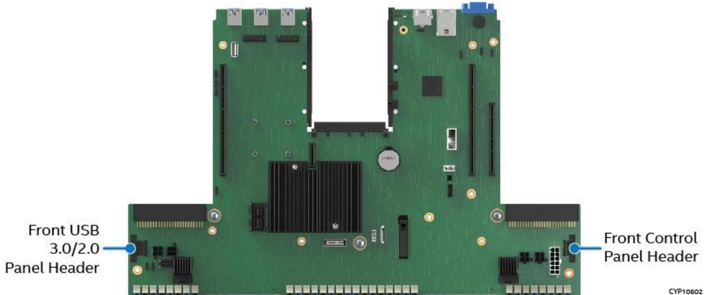
Figure 36. Front Panel Header and Front Control Panel Header
