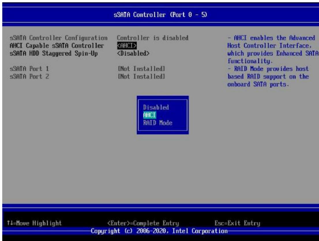
**Figure 47. BIOS Setup Mass Storage Controller Configuration Screen**
