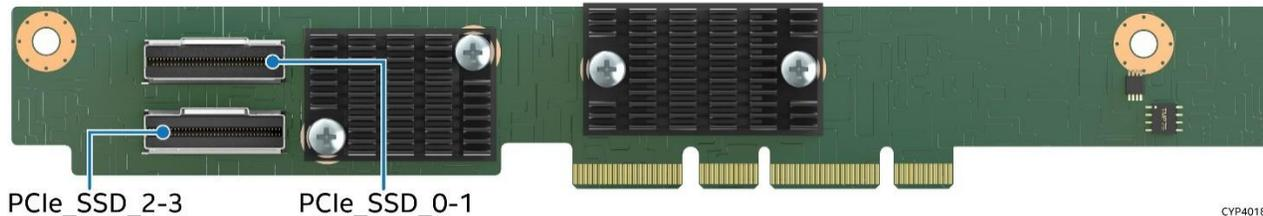
Figure 98. PCIe\* NVMe\* Riser Card for Riser Slot #3
