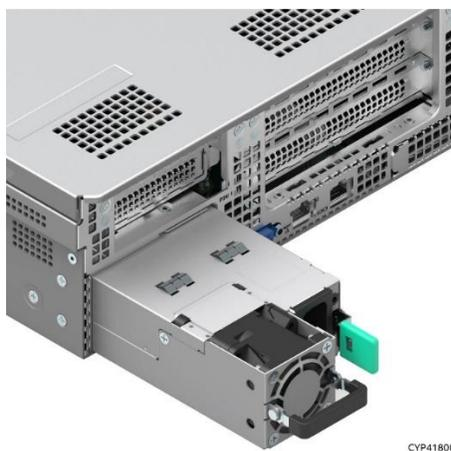
**Figure 35. Power Supply Module Partially Out of Chassis**
