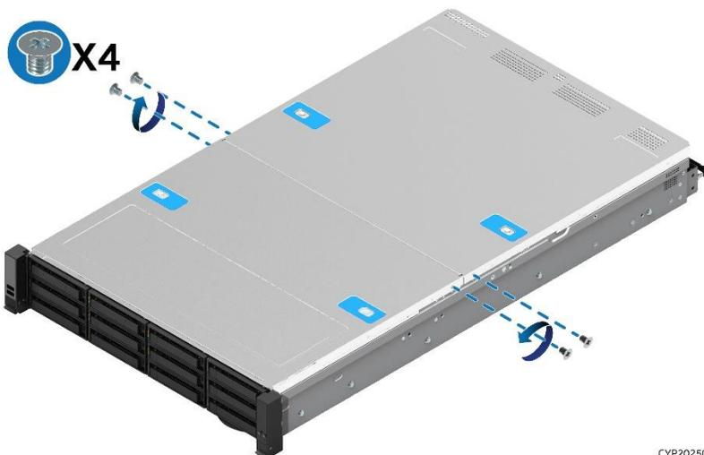
**Figure 19. Top System Cover Panels Shipping Screws**
