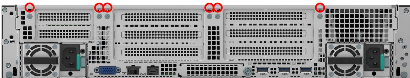
**Figure 23. Rear Panel Shipping Screw Holes**
