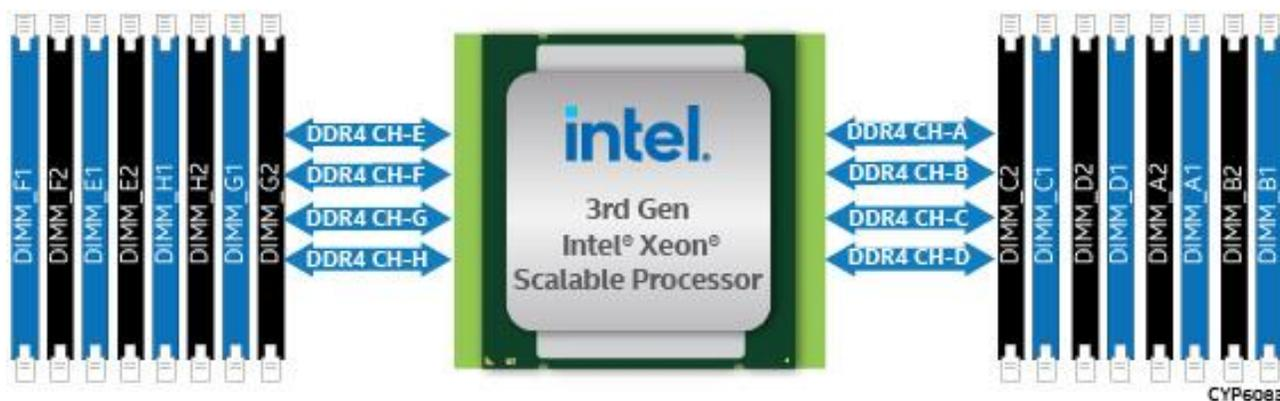
Figure 27. Memory Slot Connectivity
