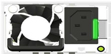
**Figure 37. AC Power Cable Connector**
