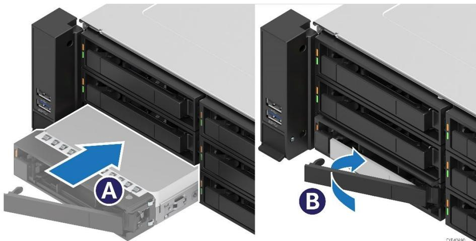
Figure 80. Drive Insertion into 3.5" Drive Bay
