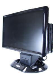
**9** Lock the monitor to the UniStand using a single M4 6mm hex socket screw.
