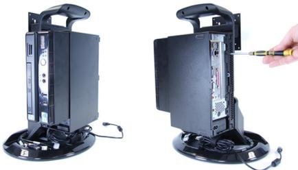
**4** Slide the Stone mini ITX computer into the receiving frame so that it sits on top of the power brick. Ensure correct orientation allowing the optical drive to open facing the user. Then secure the computer in position using two #6-32 flat head phillips screws.
