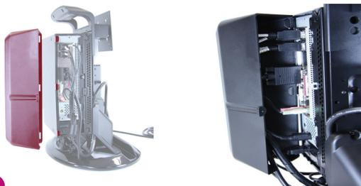
**7** Attach the cable management cover to the PC receiving frame by hooking it into position on the three protruding tabs, then rotating it on the hinged axis. Ensure that when closing the cover over the cables, no undue stress is placed on the connectors. Once fully closed, lock the cover in position with a single #6-32 hex socket screw.
