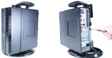
**3** Slide the Stone USFF computer into the receiving frame. Ensure correct orientation allowing the optical drive to open facing user. Then secure the computer in position using one #6-32 flat head phillips screw.
