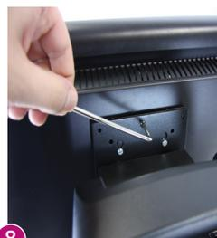
**8** Lock the monitor to the UniStand using a single M4 6mm hex socket screw.
