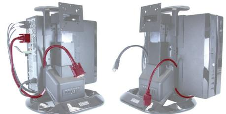
**5** Connect the supplied video cable to the video output of the computer and carefully route the cable as demonstrated in the image ensuring that it is captured behind the left hand side of the front panel in the cable recess provided.
