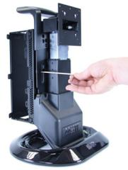
**2** Secure the PC receiving frame to the stand using one #6-32 hex socket screw in the location shown.
