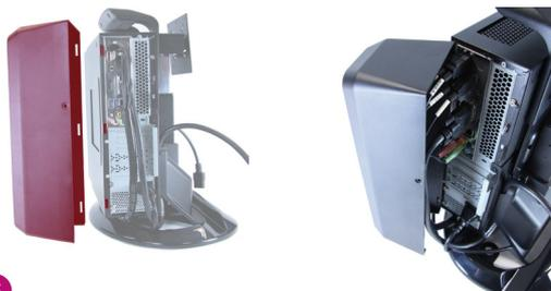
**6** Attach the cable management cover to the PC receiving frame by hooking it into position on the three protruding tabs, then rotating it on the hinged axis. Ensure that when closing the cover over the cables, no undue stress is placed on the connectors. Once fully closed, lock the cover in position with a single #6-32 hex socket screw.
