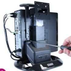
**4** Remove the two screws that retain the UniStand front panel in position.
