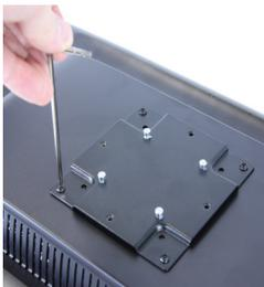
**8** Mount the VESA plate onto the rear of your monitor using four M4 9mm hex socket screws, then carefully attach the monitor to the UniStand ensuring the VESA bracket slots into position correctly.
