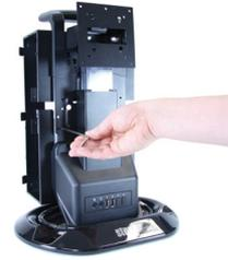
**2** Secure the PC receiving frame to the stand using two #6-32 hex socket screw in the location shown to the left and right sides of the height adjust stand.
