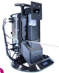
**5** Remove the two screws that retain the UniStand front panel in position.
