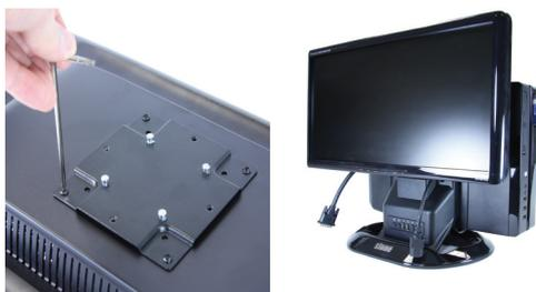
**7** Mount the VESA plate onto the rear of your monitor using four M4 9mm hex socket screws, then carefully attach the monitor to the UniStand ensuring the VESA bracket slots into position correctly.
