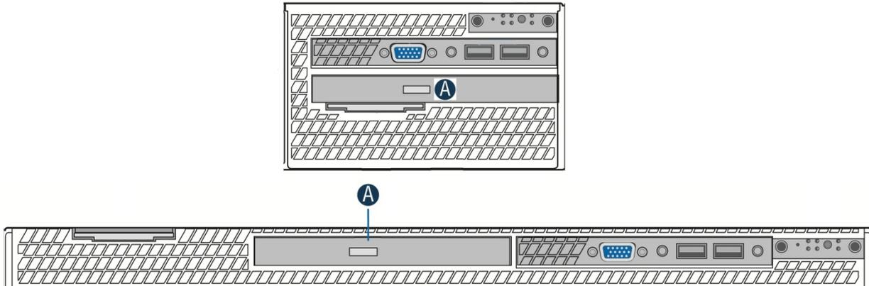
**Figure 32. Optical Drive Support**
