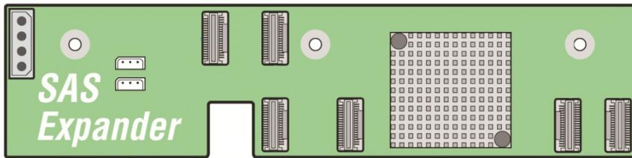
**Figure 40. Internal 24-Port SAS Expander Card (RES2CV240)**
