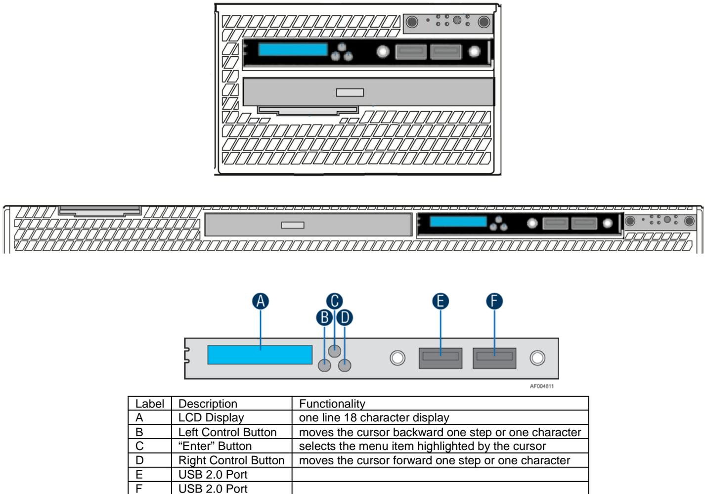
**Figure 46. Intel Local Control Panel Option**
