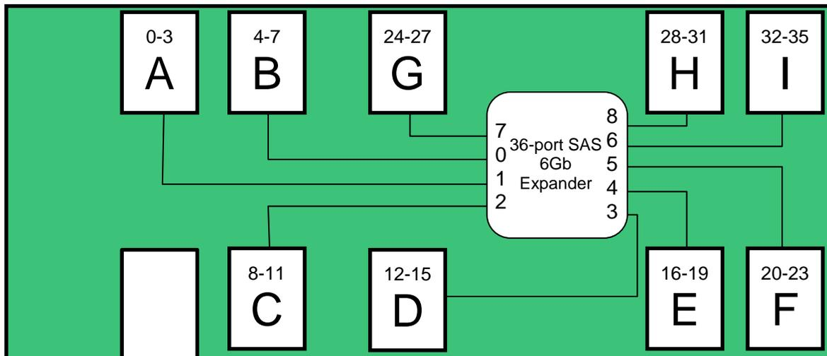
Figure 43. 36-Port Expander SAS Connector/Drive Identification Block Diagram
