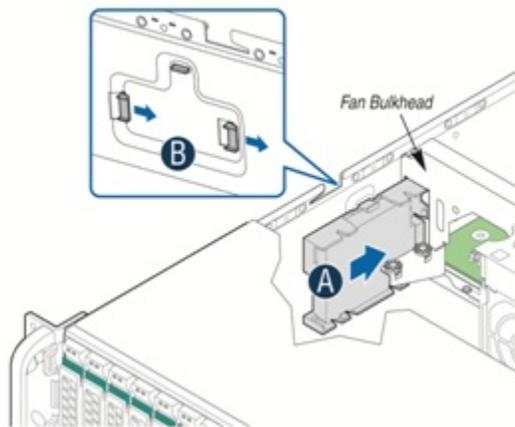
Figure 36. AXXBBU9 Installation
