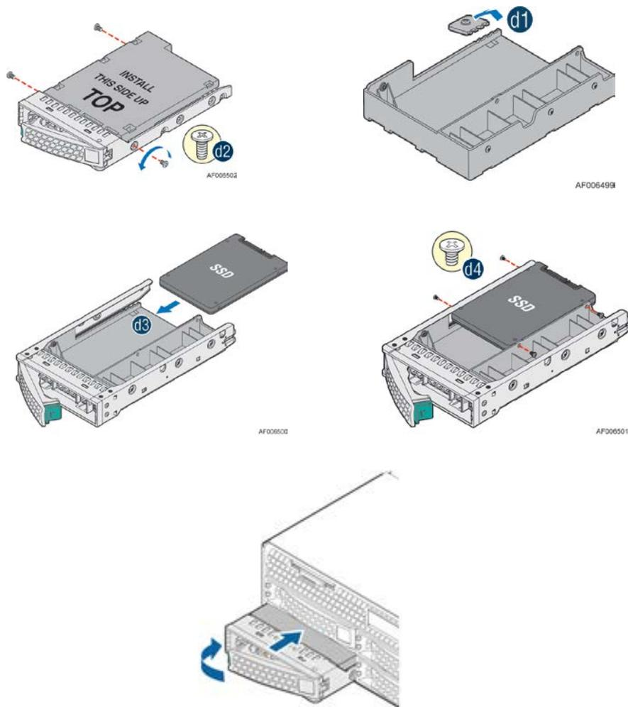
Figure 31. Option to install 2.5" SSD into a 3.5" drive blank
