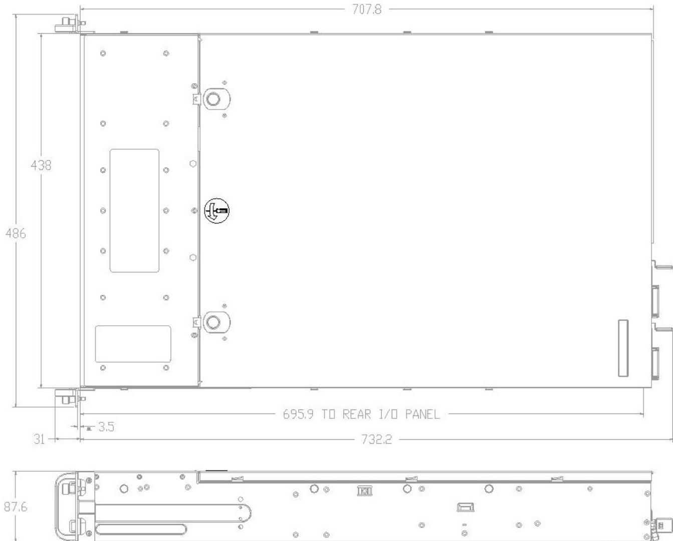
**Figure 1. Chassis Dimensions**
