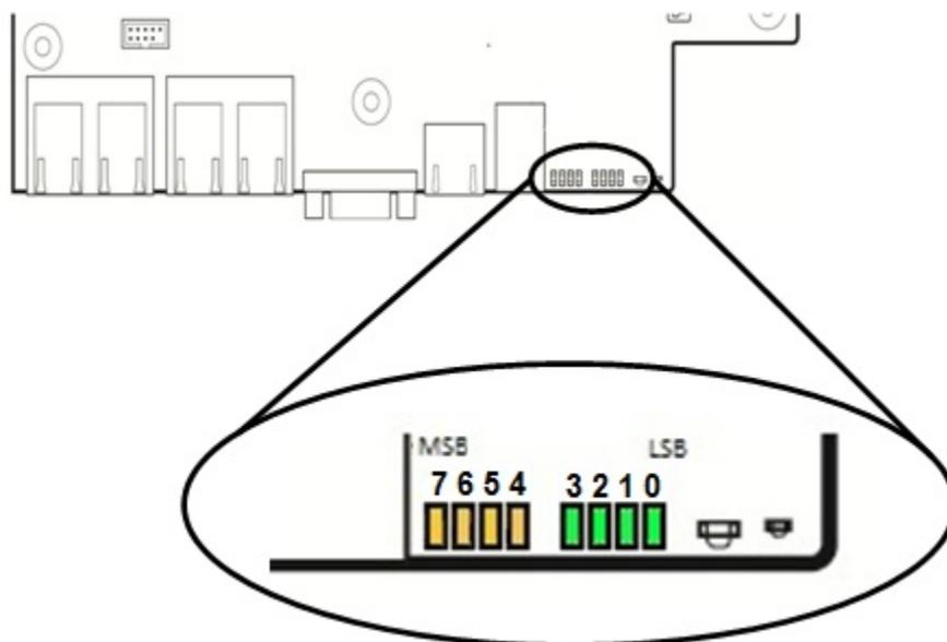
Figure 53. POST Diagnostic LED Location
