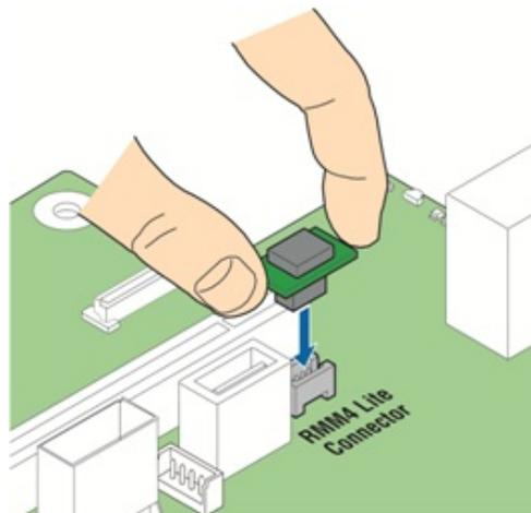
Figure 52. Intel® RMM4 Lite Activation Key Installation
