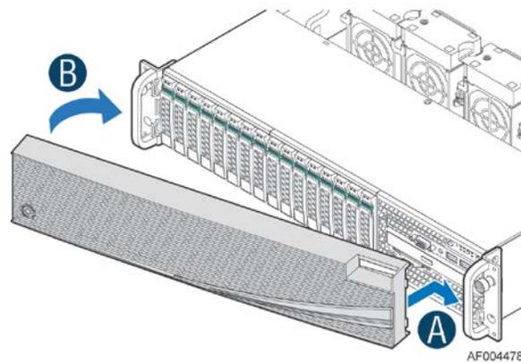
The face of the bezel assembly includes snap-in identification badge options and a wave feature option to allow for customization.
