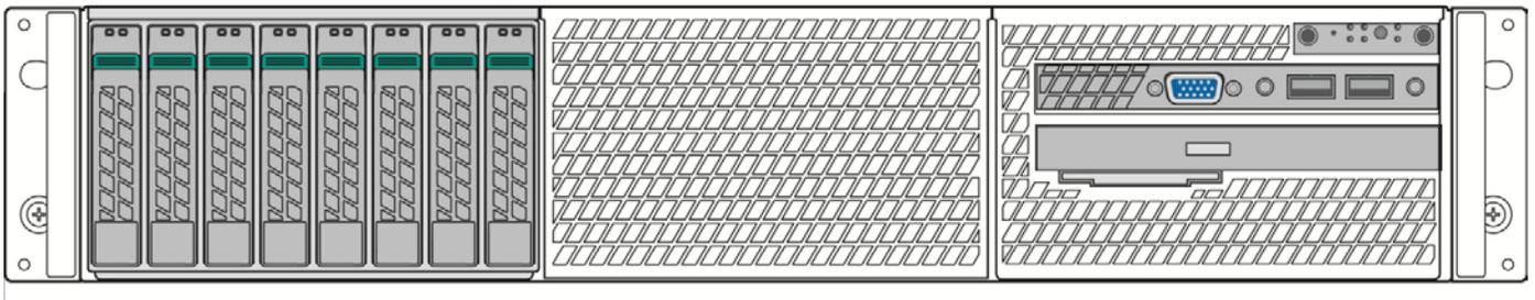
**Figure 5. 2.5" Hard Drive Bay - 8 Drive Configuration**
