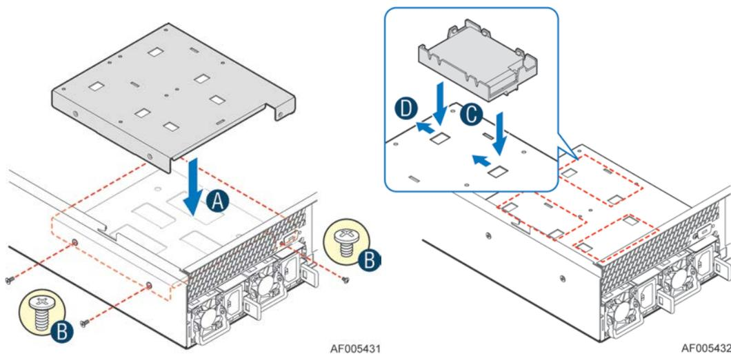
Figure 37. A2UBKTMFBUSSD Bracket + AXRMFBU2 Installation
