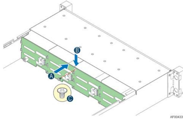
On the front side of each back plane are mounted eight or twelve hard disk drive interface connectors, each providing both power and I/O signals to attached hard disk drives.
