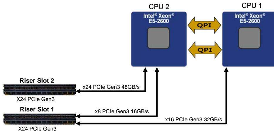
Figure 47. Riser Slot Architecture
