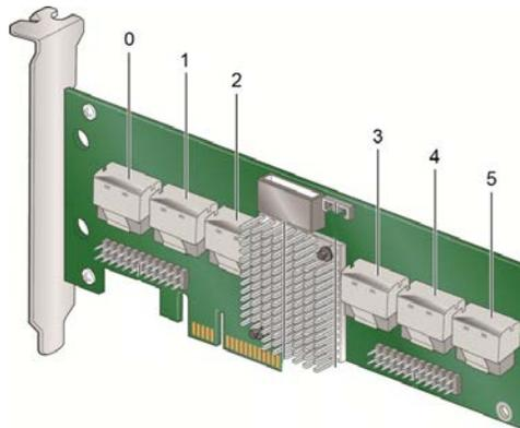
**Figure 38. 24 Port PCIe Intel® RAID Expander Card RES2SV240**
