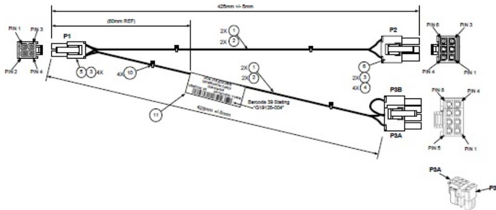
The power cable (as shown above) for the OPT\_12V\_PWR\_# connector is included in the 2-slot Riser Card accessory kit (A2UL16RISER ) and can support both 6 and 8 pin GPU card 12V AUX power connectors.
