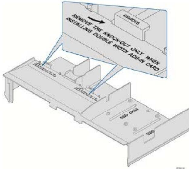
Figure 26. Intel Accessory Kit AGZCOPRODUCT - Air Duct
