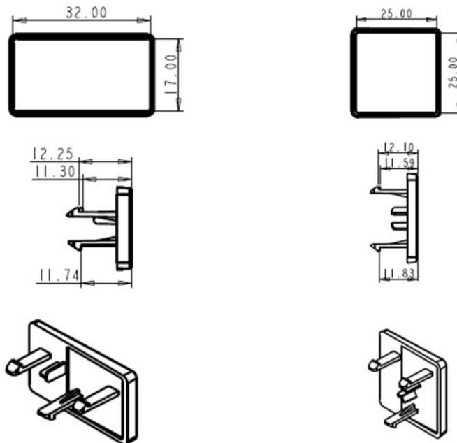
Figure 15. Front Bezel accessory ID Badge mechanical drawings
