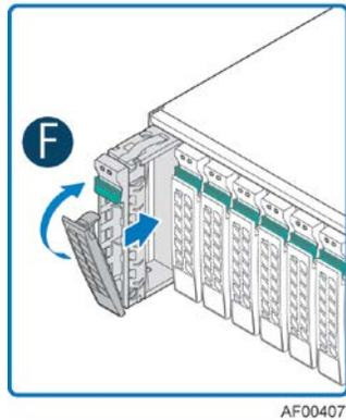
**Note: To maintain system thermals, all drive bays must be populated with a drive tray mounted with a hard drive, SSD, or supplied drive blank.**
