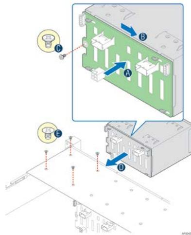
On the front side of each backplane are mounted eight storage device interface connectors (A), each providing both power and I/O signals to attached storage device.
