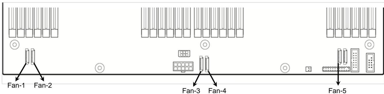
**Figure 25. Server Board System Fan Connector Locations**
