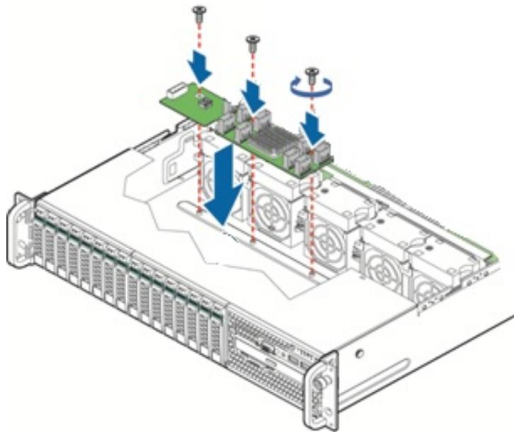
**Figure 39. Internal SAS Expander Installation**
