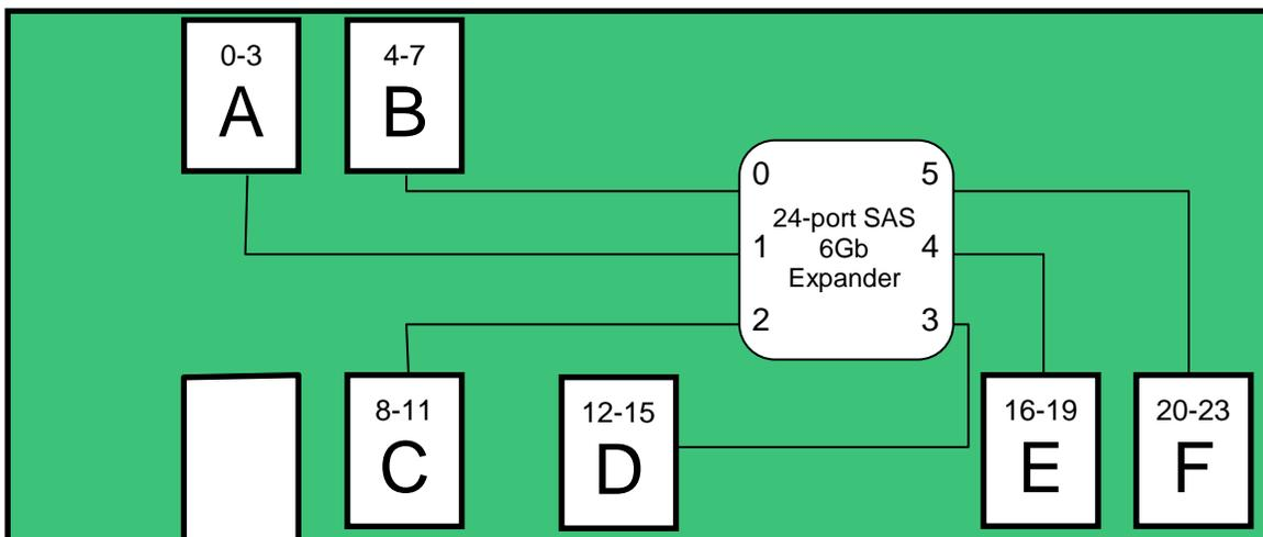
**Figure 41. 24-Port Expander SAS Connector/Drive Identification Block Diagram**
