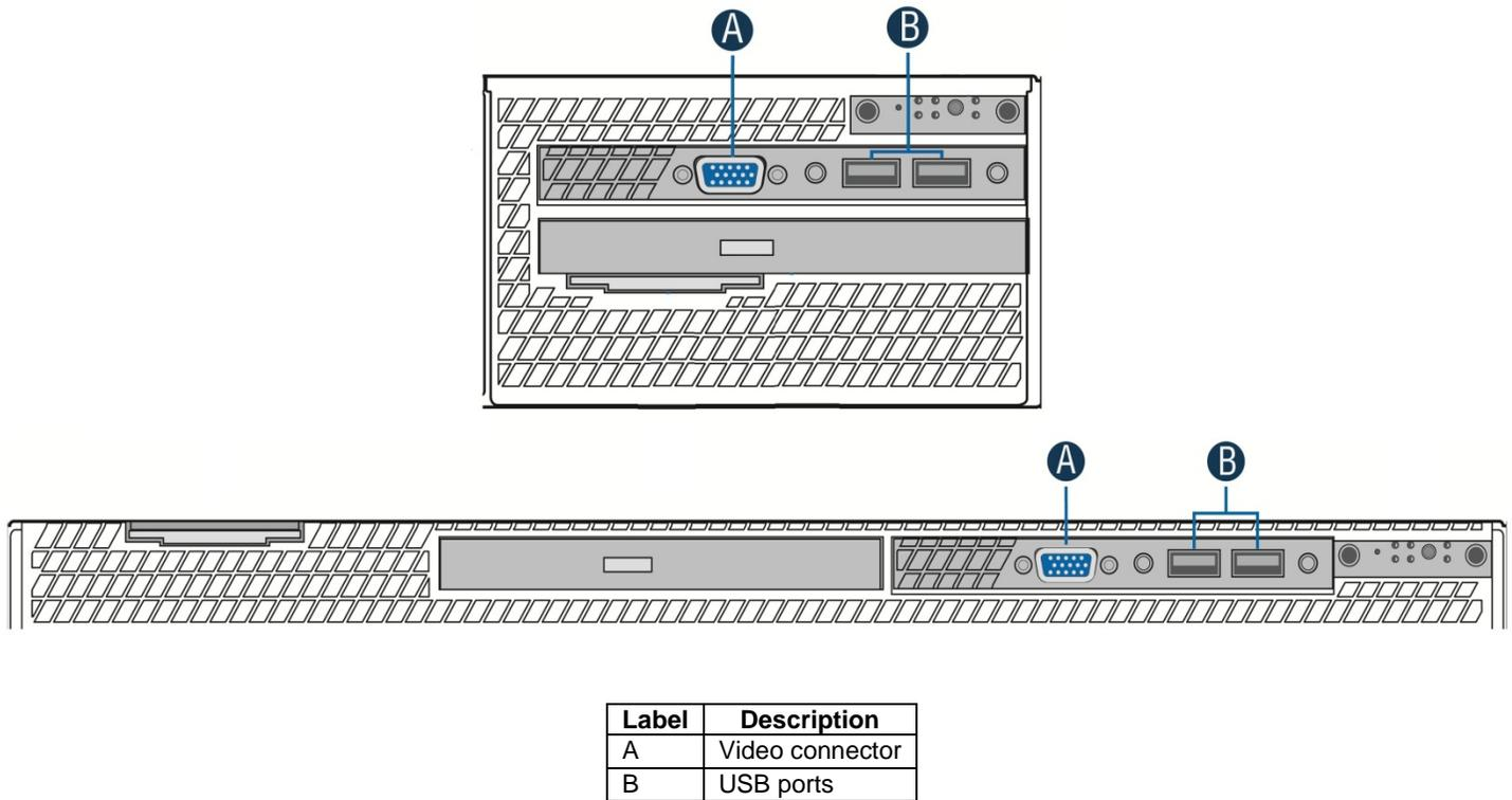
**Figure 44. Front I/O Panel Features**
