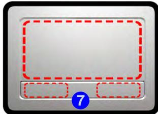
Note that the Touchpad and Buttons has a valid operational area indicated within the dotted lines above.
