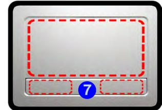
Note that the Touchpad and Buttons has a valid operational area indicated within the dotted lines above.
