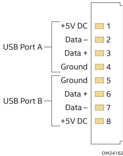
**Figure 15. Connection Diagram for Internal USB 2.0 Dual-Port Header (1.25 mm Pitch)**
