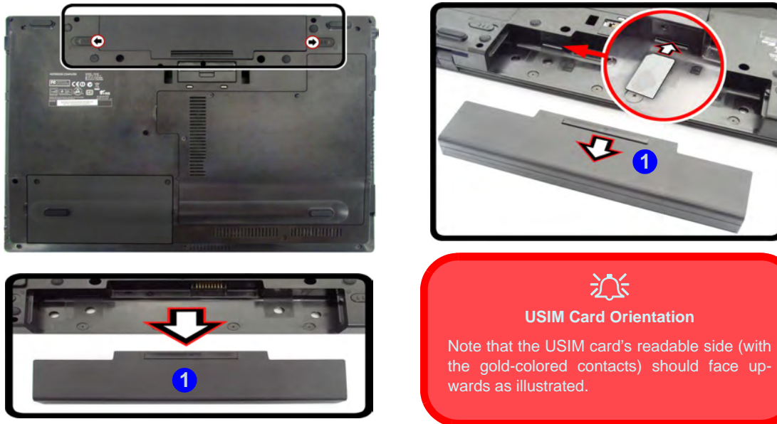
Figure 5 - Battery Removal & USIM Card Insertion
