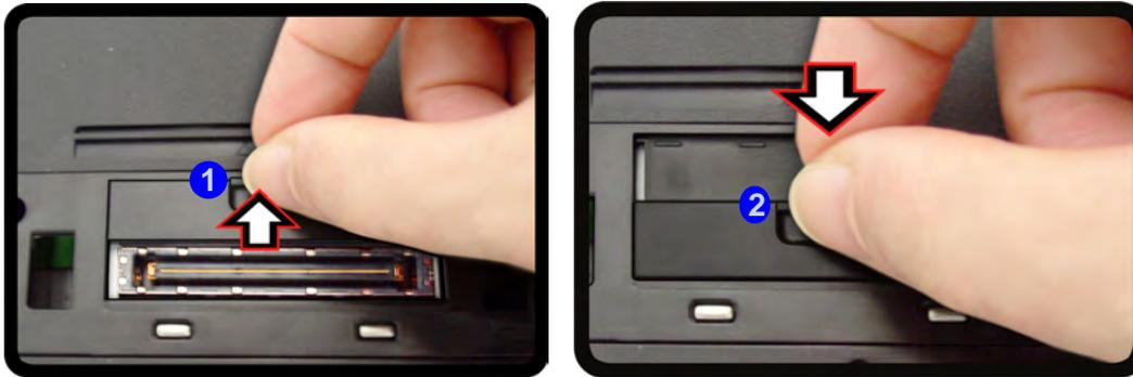
Figure 1 - 8 - Opening and Closing the Docking Port
