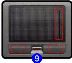
Note that the valid operational area for the Touchpad's scroll bar and Buttons is that indicated within the red dotted lines above.
