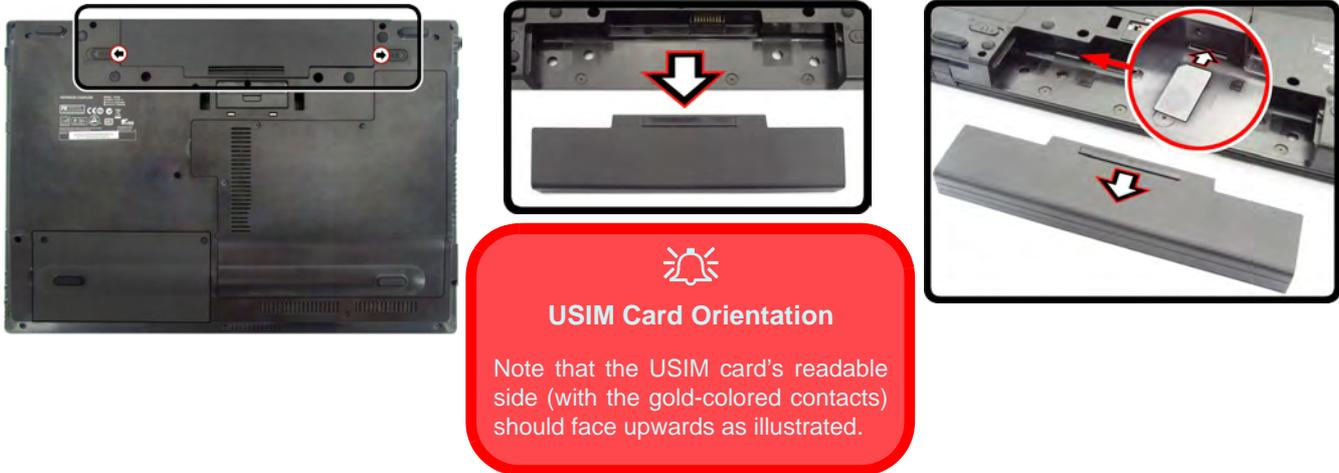
Figure 1 - 7 - Battery Removal & USIM Card Insertion
